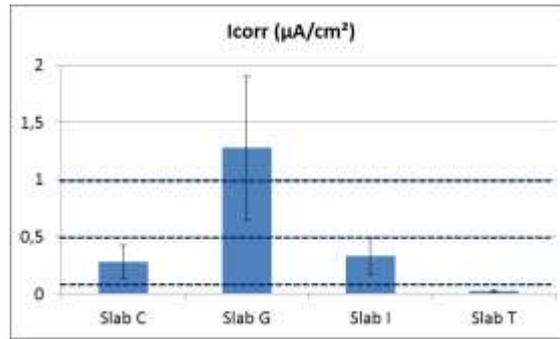
Figure 4. Average corrosion current density values per slab. The corrosion level thresholds recommended by the RILEM (8) appear in blue-dotted-lines
