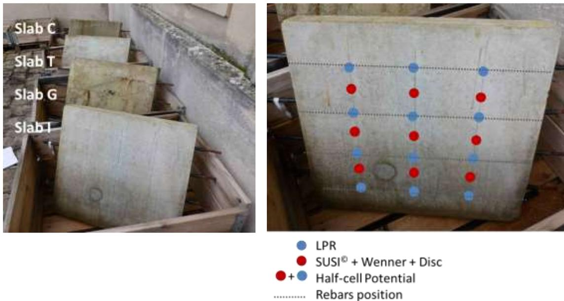
Figure 1. Four specimens considered and implementation of the testing protocol.
