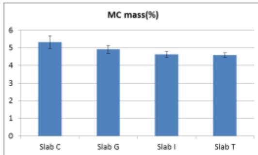
Figure 5. Average mass moisture content per slab.
