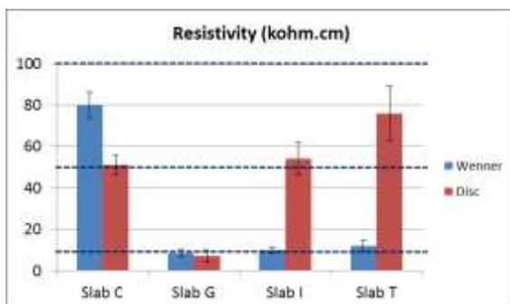
**Figure 2. Average resistivity. The corrosion risk thresholds recommended by the RILEM (6) appear in blue-dotted-lines**
