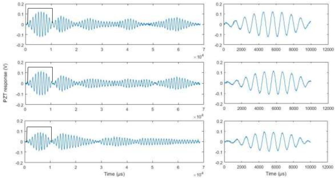
**Figure 2: Left: Three high-passed PZT responses at different stages of the fatigue loading (top: begin; middle: middle; bottom: end) and the selected time gate. Right: The same signals after time gating.**
