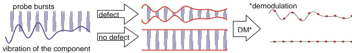
**Figure 1. General concept of the developed crack detection method: the vibration of the component opens and closes a crack and thereby modulates the probe waves. In the absence of a crack no modulation is detected**
