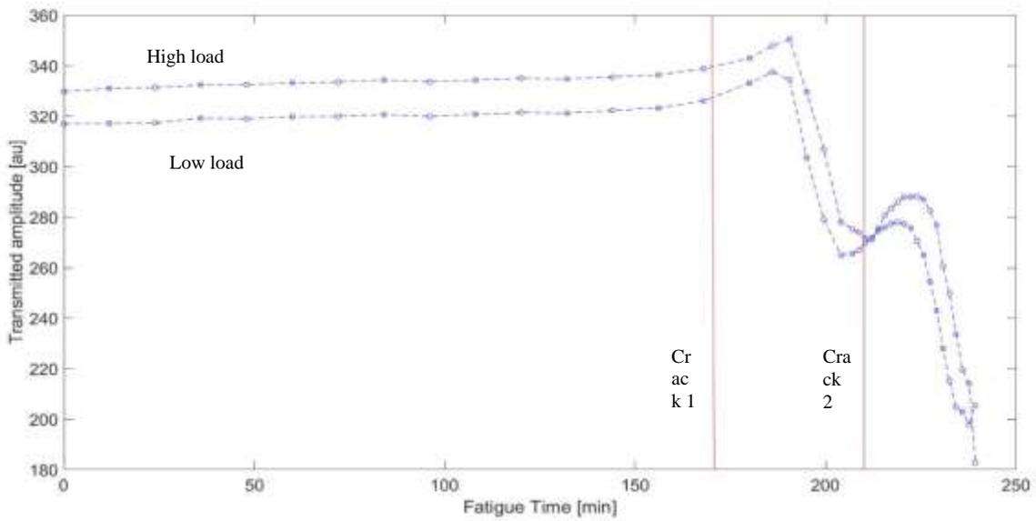
Figure 4: Transmission amplitudes versus fatigue loading time .
