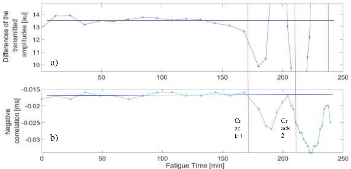
**Figure 5: Illustration of defect detection thresholds based on two tentative diagnostic algorithms: a) difference between transmitted amplitudes at high/ low - load conditions versus fatigue time b) negative correlation analysis versus fatigue time.**
