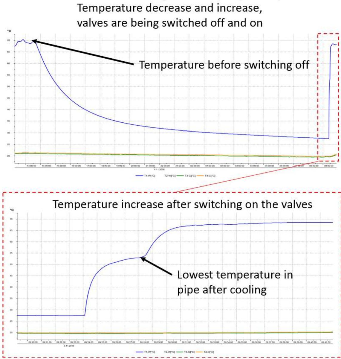
**Figure 4. The top graph shows the cooling phase start at about 69 °C. The lower graph shows the lowest temperature in pipes after cooling down and switching on, in this case 53 °C.**
