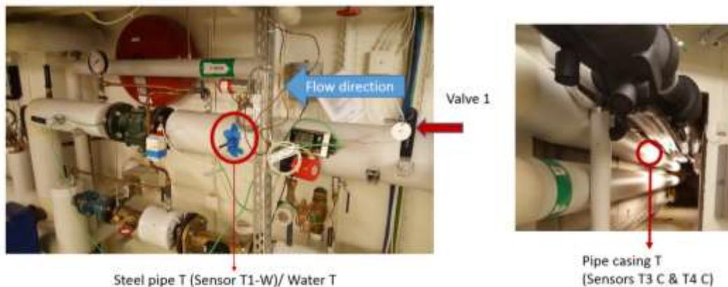
**Figure 3. Experimental setup of the cooling method on Chalmers pipes. The steel pipe sensor is located to the left of the enclosed water volume and 0.3 meter to the right of the uninsulated connections.**
