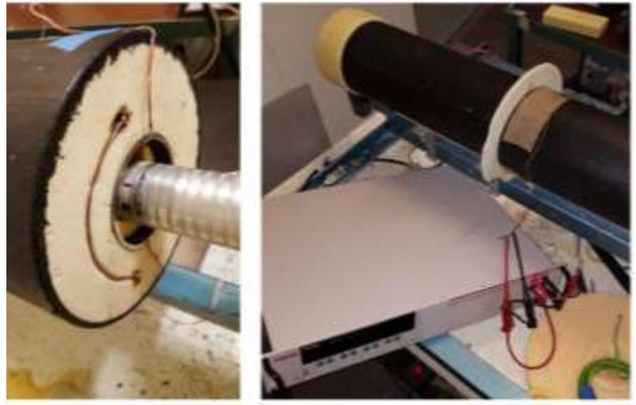
Figure 1. Test setup for resistance measurement while using the GHP method
