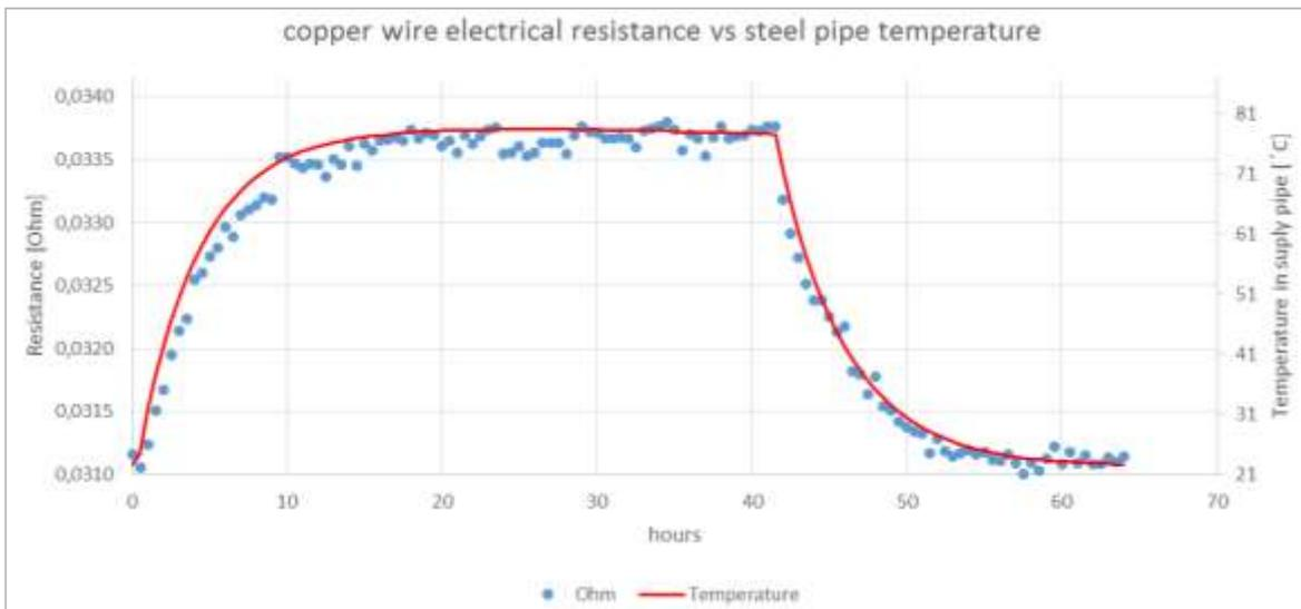
Figure 2. Steel pipe temperature (water temperature) and electrical resistance. The graph shows a clear connection between the temperature in red and the resistance in blue.
