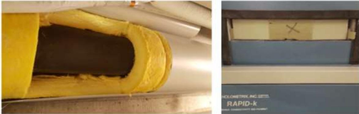
**Figure 5. The picture to the left shows the pipe with the removed insulation piece. The image to the right shows parts of the removed insulation when tested using the guarded heat flow meter.**
