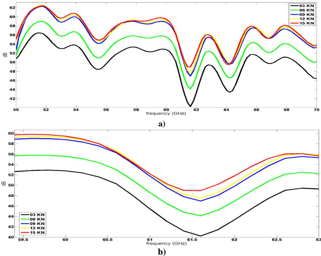
**Figure 5: Measured reflection a) in the range 50-70 GHz electromagnetic radiation and b) around 61.5 GHz electromagnetic radiation**
