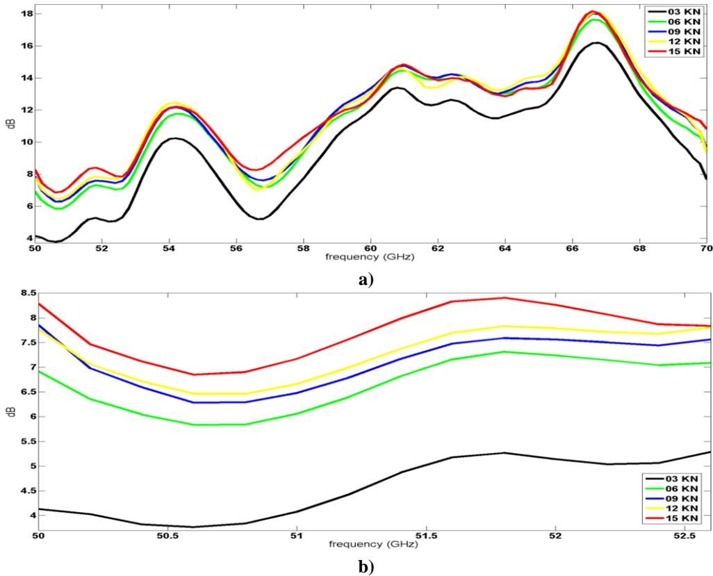
Figure 6: Measured transmission a) in the range 50-70 GHz electromagnetic radiation and b) around 51.5 GHz electromagnetic radiation
