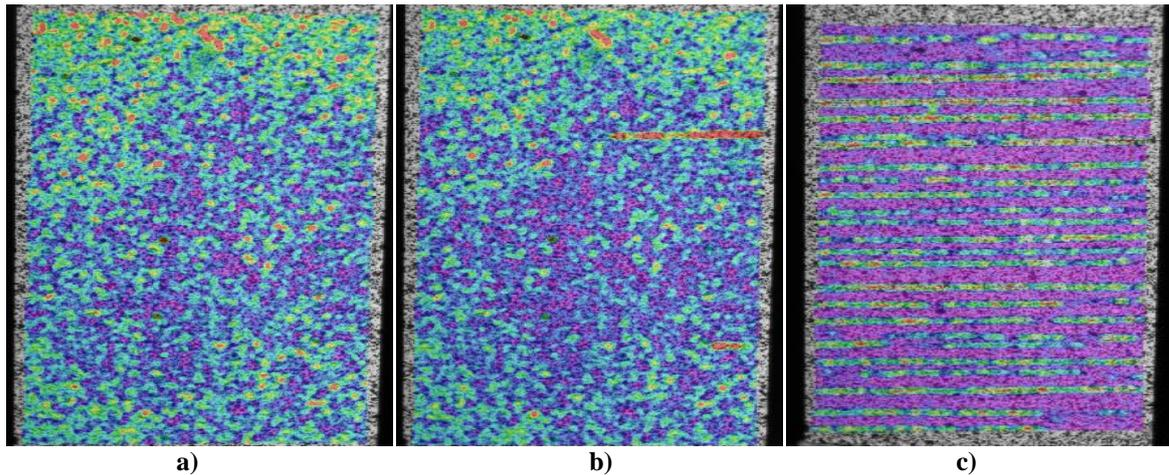
**Figure 3:**  $\sigma$  value map obtained from DIC at a) 70 MPa, b) 100 MPa and c) 330 MPa stress
