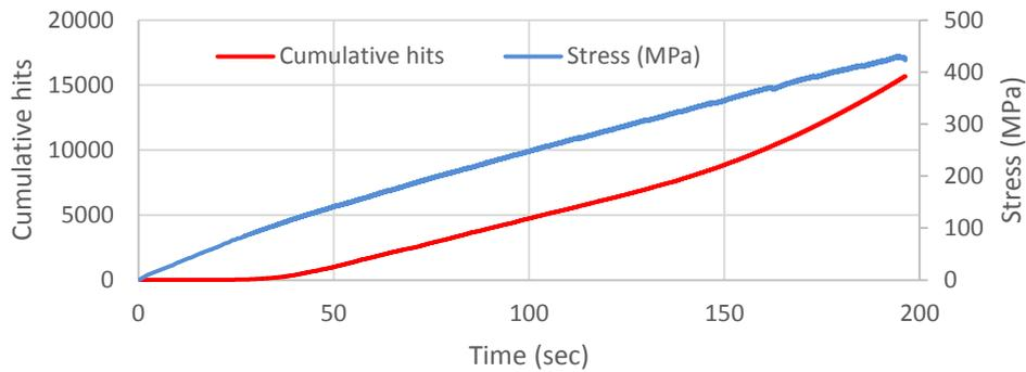
**Figure 2: Evolution of the AE activity and the stress during static tests**
