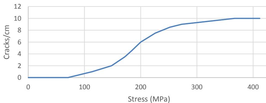
**Figure 4:** Evolution of the crack density as a function of the applied stress
