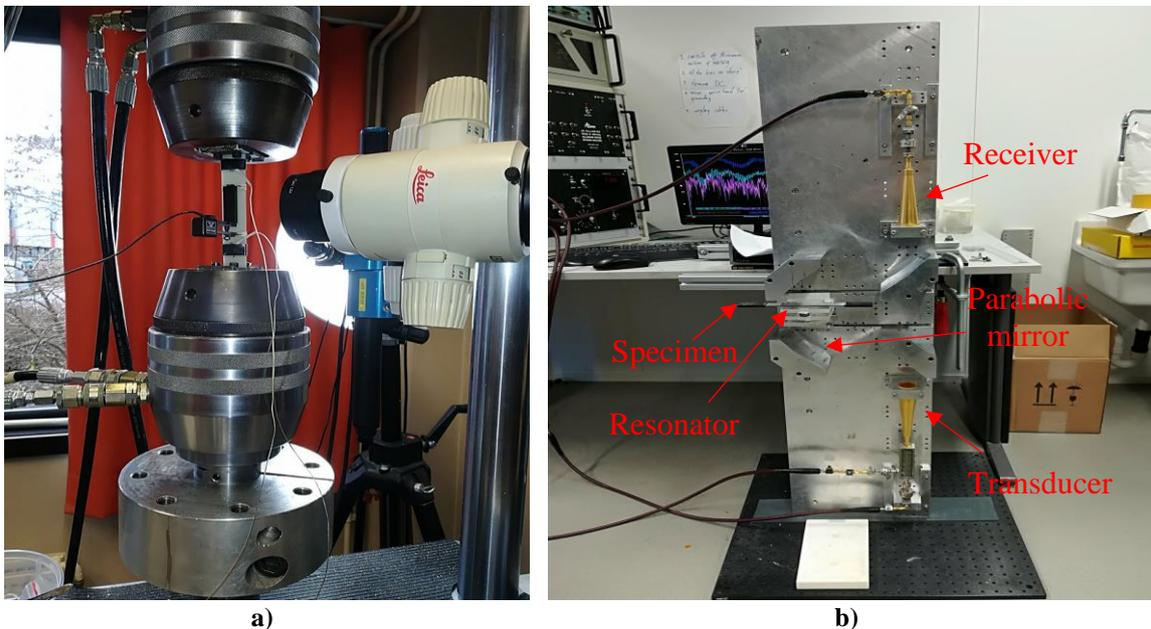
Figure 1: a) Set-up used for testing and b) MMW equipment used
