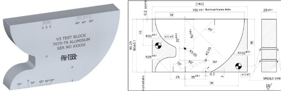
**Figure 2. V3 calibration block proposed for nonlinear NDT standards. Instead of using V1 calibration block known for its regular geometry, V3 is preferred because complex propagation increases the reverberant properties needed for TR-NEWS focusing.**
