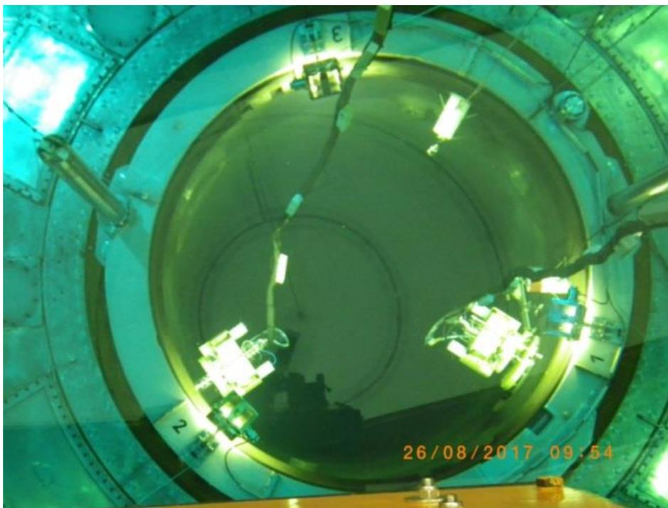
**Figure 3** *Inspection of Inlet and Outlet Nozzle to Shell welds with two manipulators working in parallel*
