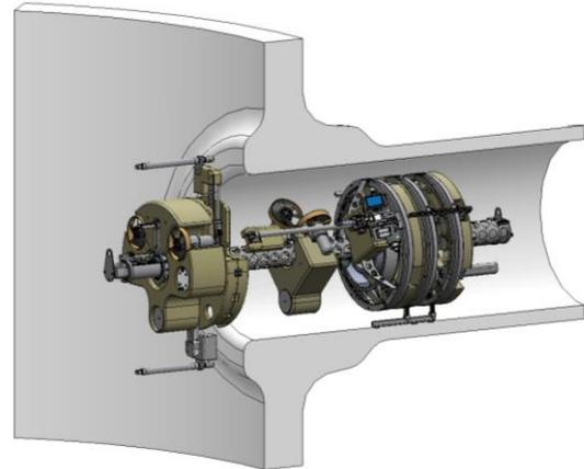
**Figure 1** Different Grotte configurations for inspection of the In- and Outlet nozzles
