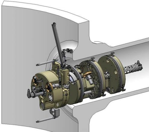
Grotte Configuration for inspection of Outlet Nozzle from the Nozzle Bore
