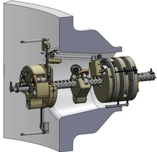
Grotte Configuration for inspection of Outlet Nozzle from the RPV wall
