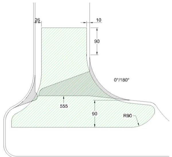
**Figure 2** Inspection Volume for Inlet and Outlet Nozzle to Shell Welds
