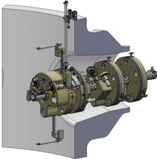
Grotte Configuration for inspection of Inlet Nozzle from the Nozzle Bore
