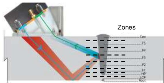
Figure 1. Inspection set-up.
