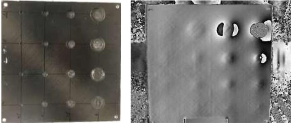
Figure 2. Sample with drilled bottom holes (left) and measured phase map (right)
