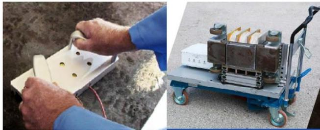
**Figure 4. MsT (left) and EMAT (right) for guided wave inspection of containment vessels**
