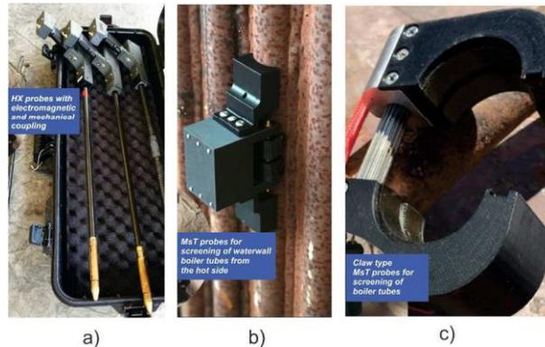
**Figure 8. Ruggedized MsT probes: a - for GWT of HX tubing with electromagnetic and mechanical coupling, b – for GWT of water-wall boiler tubing, c - claw type probe for GWT of boiler tubing.**
