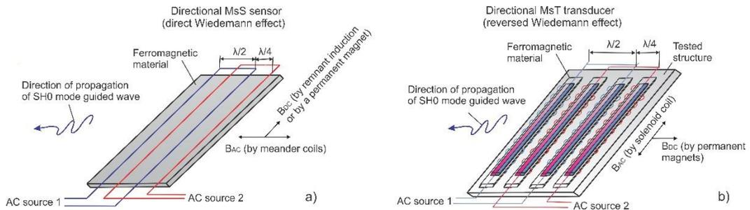
**Figure 3. Directional transmission of guided waves: a – utilizing two quarter wavelength spaced meander coils (each coil has two conductors separated by half of the wavelength); b – utilizing two quarter wavelength spaced MsT transducers (each transducer has two channels separated by half of the wavelength, connected to reject the unwanted direction).**
