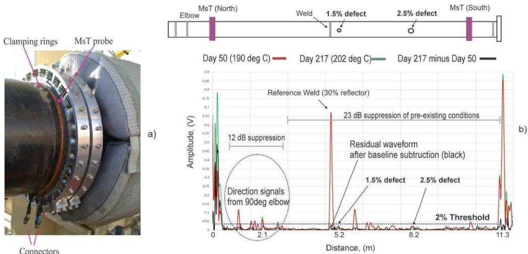
**Figure 5. Results of MsT testing on 219 mm OD schedule 40 pipe: a – probe setup with bonded MsT and a retention clamp, b – overlapped A-scan traces at day 50 at 190°C (red) and day 217 at 202°C (green). Results of baseline subtraction are shown in black.**
