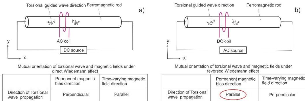
**Figure 1. Two alternative implementations of Wiedemann effect: a – direct Wiedemann effect when the circumferential field is permanent and b - a reversed Wiedemann effect when the circumferential field is time-varying.**
