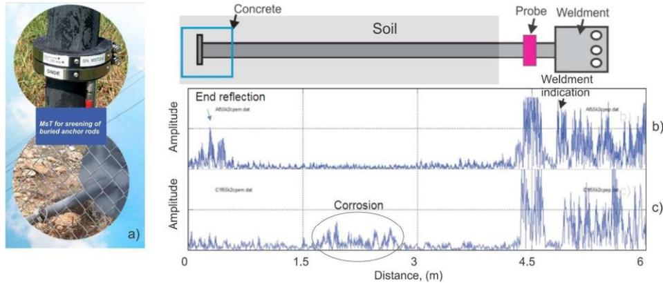
**Figure 7. Testing of buried anchor rods using MsTs: a – a transducer dry coupled to 56 mm OD anchor rod, b – data acquired from a buried anchor in good condition at 50 kHz, c – data acquired from an anchor with localized corrosion at 50 kHz.**
