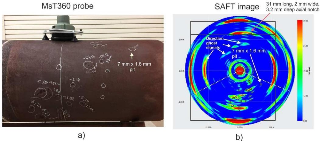
**Figure 6. a- MsT 360 probe mounted on top of a 609 mm OD, 7 mm wall carbon steel pipe, b – SAFT imaging of tested structure using 150 kHz shear horizontal guided waves.**
