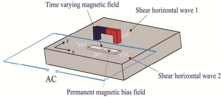
**Figure 2. A configuration to generate shear waves propagating in orthogonal directions using two orthogonal magnetic fields.**
