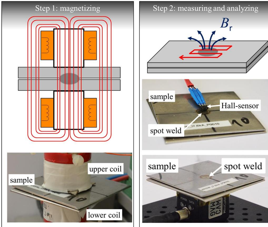
**Figure 2. Testing procedure and experimental setup with magnetizing coils, Hall-sensor and Magcam Minicube1D**
