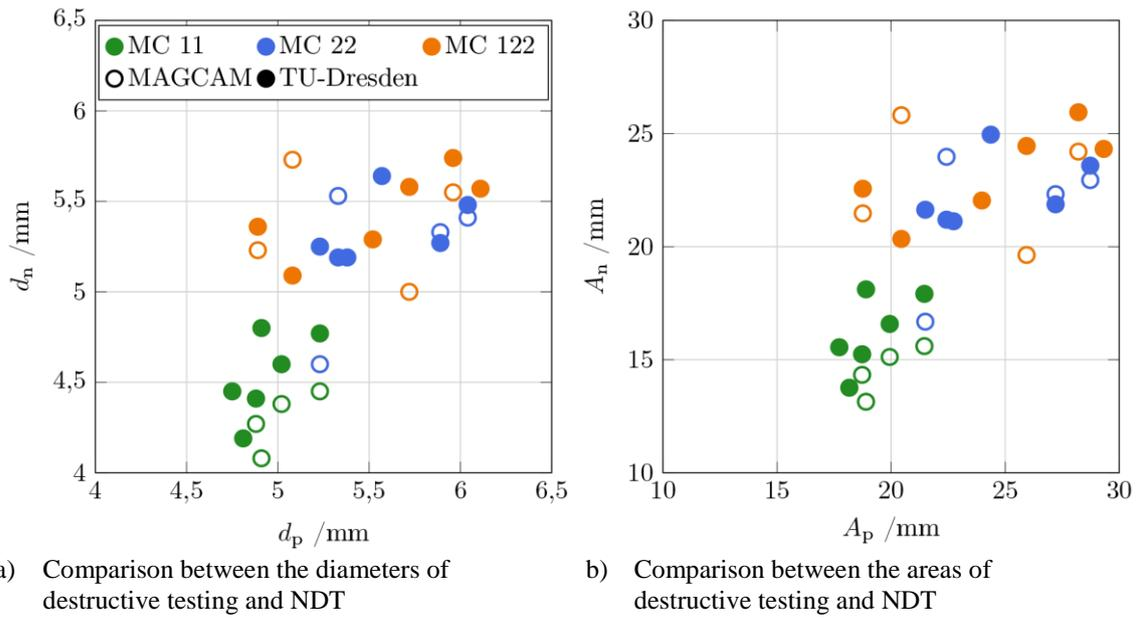
**Figure 5. Comparison of destructive testing ( $d_p, A_p$ ) vs. NDT ( $d_n, A_n$ ) used the experimental setup with Hall-sensor (TU-Dresden) and the magnetic field camera Magcam Minicube1D (MAGCAM)**
