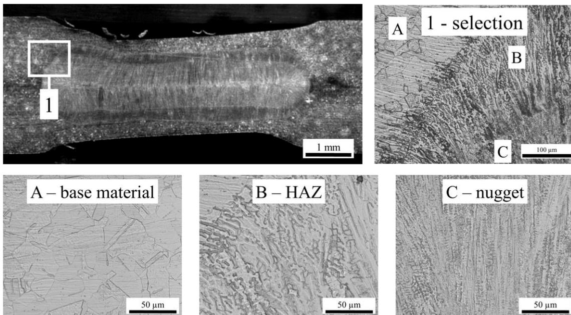
**Figure 7. Microstructure of a spot weld with two 1.4301 (1,5 mm) (pictures taken by [9])**
