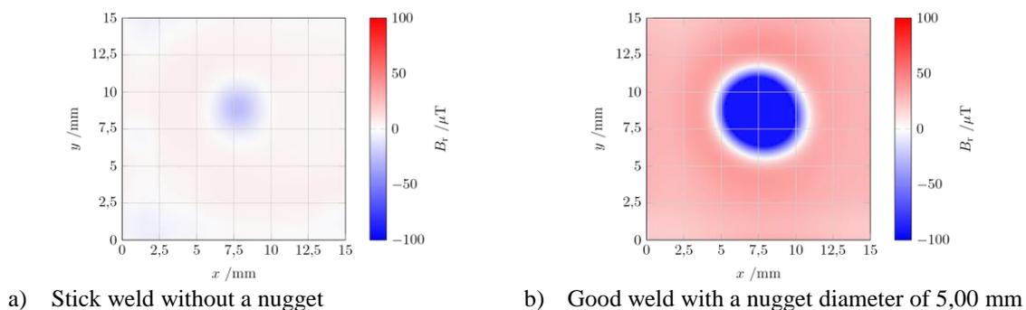
**Figure 4. Different NDT measurement results cause by different spot welding qualities**
