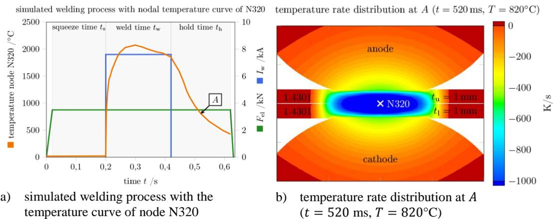
**Figure 6. Temperature development and rate distribution of the welding process of MC 11, PS3 simulated with SORPAS 2D R12.5 ( $F_{el} = 3,5 \text{ kN}$ ,  $t_w = 220 \text{ ms}$ ,  $I_w = 7,6 \text{ kA}$ )**
