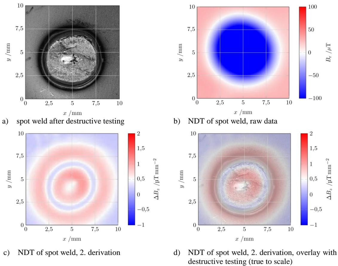
**Figure 3. Comparison and overlay of a destroyed sample with the NDT measurement results and analysis algorithm**
