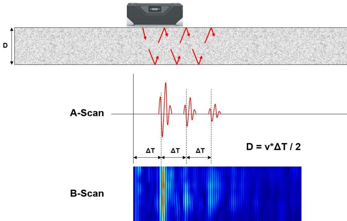
**Figure 4. Pulse-echo measurement principle. The depth is calculated from the transmission time and the pulse velocity**
