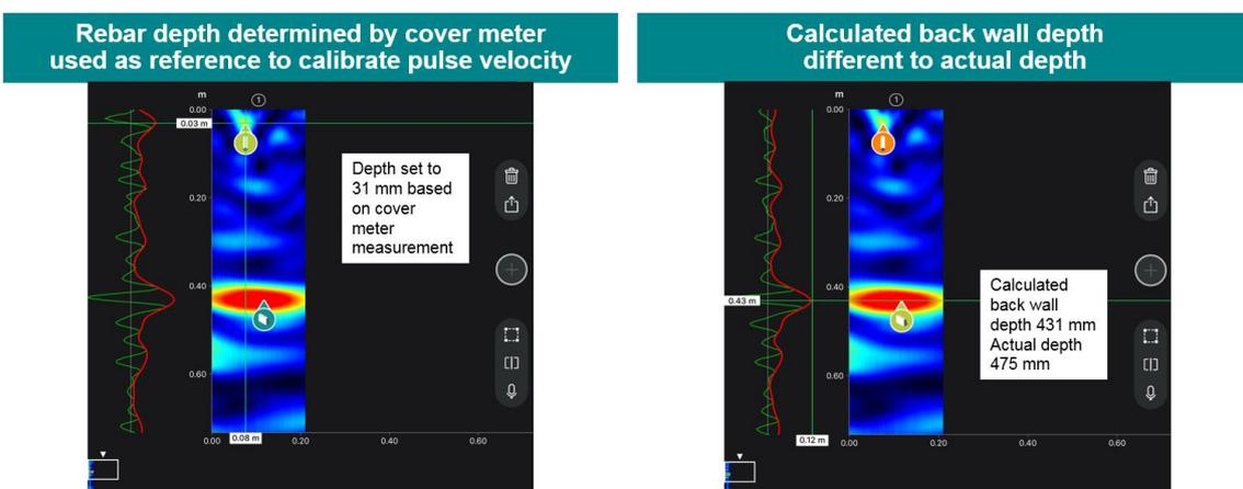
**Figure 6. Pulse-velocity calibration using reference rebar depth. The depth of the rebar is accurately determined using a cover meter. This is used to calibrate the pulse velocity, which in turn is used to calculate the depth of other objects, such as the back wall**
