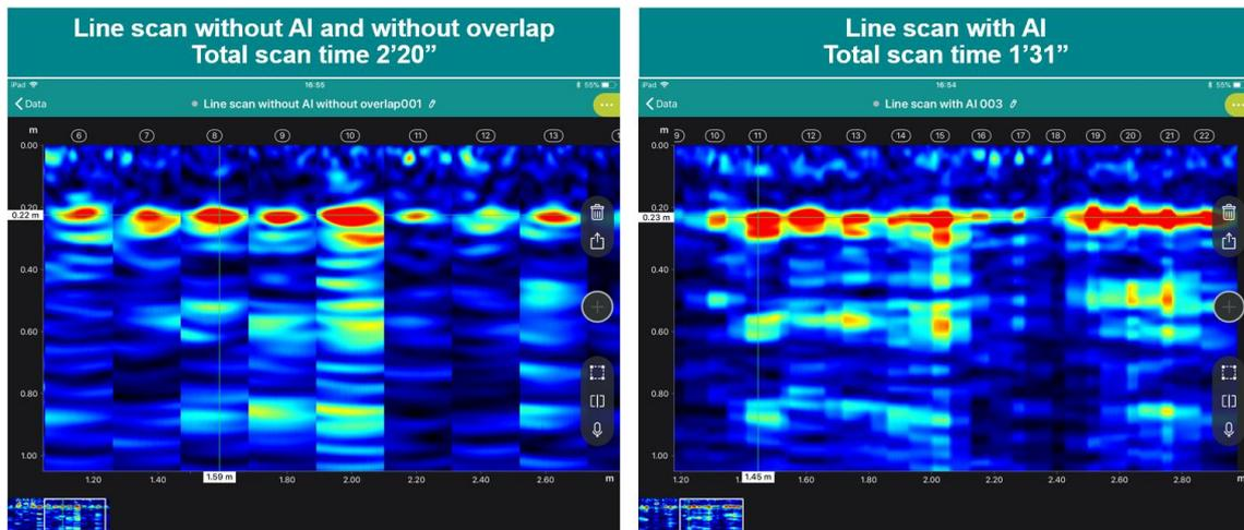
**Figure 1. Large scale scans with and without the use of intelligent positioning.
