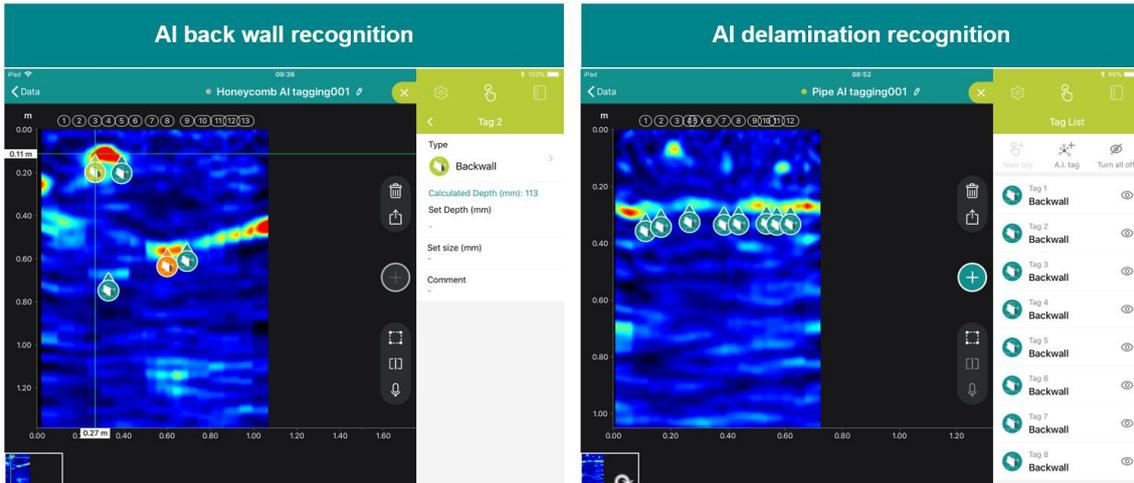
**Figure 3. A.I.-assisted object recognition of smaller objects. The B-scan on the left shows a scan of a V-shaped concrete element with honeycombing close to the surface. The B-scan on the right shows a concrete element, 30 cm thick, with three hollow pipes.**
