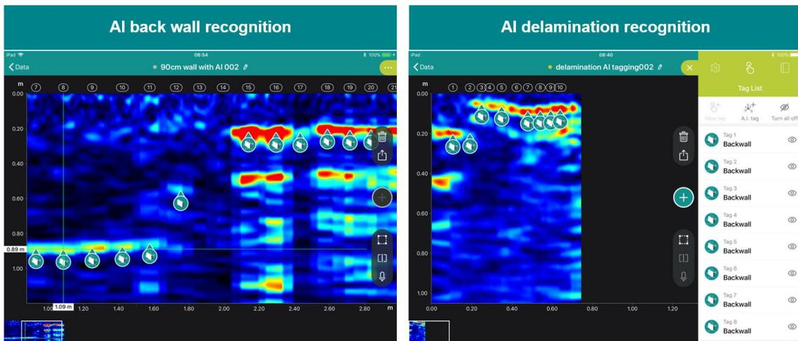
**Figure 2. A.I.-assisted object recognition. The B-scan on the left shows tagging of a back wall with a step change of 70 cm in thickness. The B-scan on the right shows tagging of a large delamination.**
