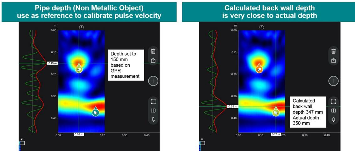
**Figure 5. Pulse-velocity calibration using a reference pipe depth. The depth of the pipe must be determined by another technology (in this case, GPR). This is used to calibrate the pulse velocity, which in turn is used to calculate the depth of other objects, such as the back wall**
