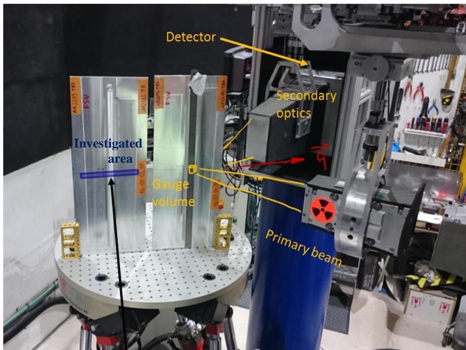
**Figure 1** Set-up for measurements in two test welds at the same time. The primary beam is shaped by two radial focussing collimators. A third collimator (secondary optics) in front of the detector defines the third dimension of the gauge volume (here  $0.6 \times 0.6 \times 2 \text{ mm}^3$ ).
