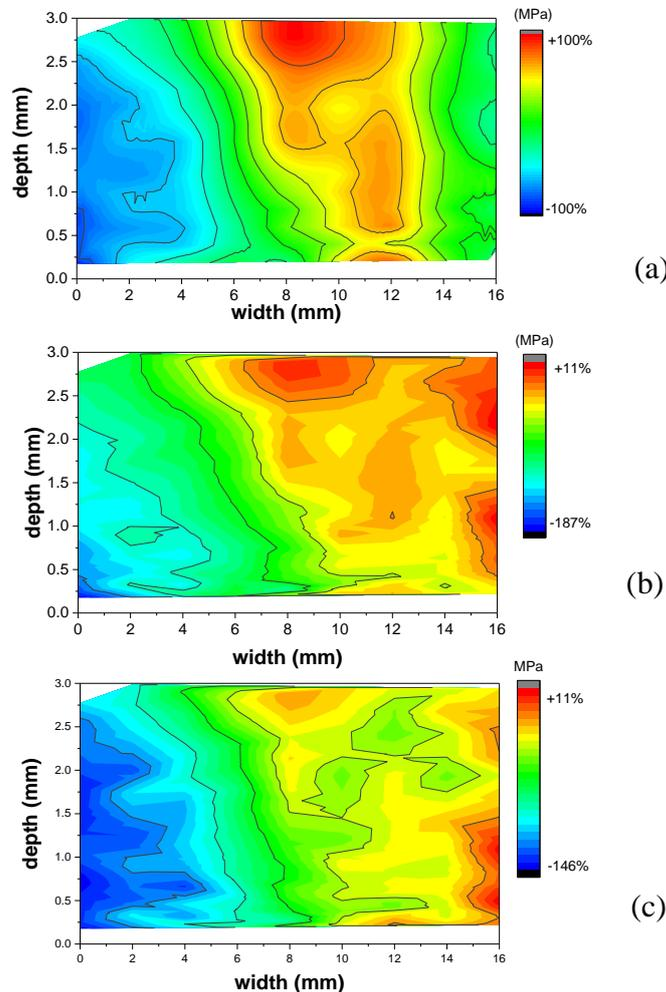
**Figure 2 Residual stress 2D mapping and depth profiles of (a) longitudinal (b) transversal and (c) normal components.**
