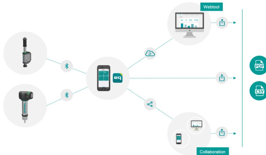
**Figure 4: The Proceq Live ecosystem diminishes manual data entry and reporting effort and enables real-time data sharing and collaboration between users. Transducers are connected via wi-fi to the mobile device, which connects to the data backup system wirelessly via WLAN or 3G/4G. Reports, webtool access and collaboration options are facilitated.**
