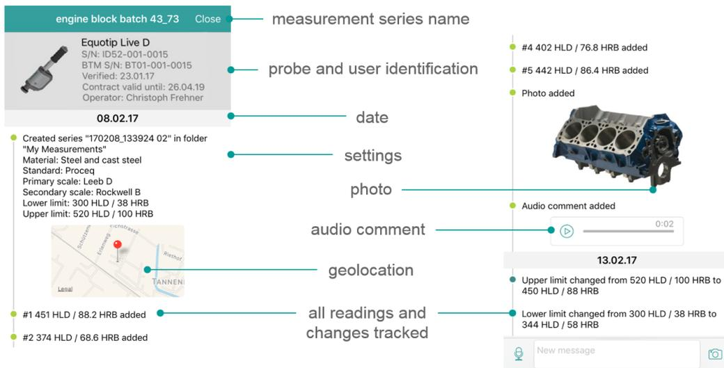
**Figure 3: Logbook example of a Proceq Live product which tracks the measuring process. The comprehensive Logbook describes the device and names the user, it logs settings and measurement parameters, and records readings and exclusion of readings. Moreover, it permits adding photos and notes.**
