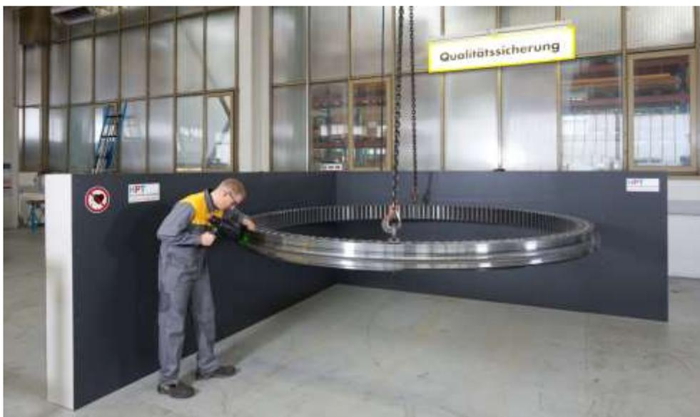
Figure 3: Non-contact MT-testing and demagnetization of a gearwheel carrier with an approx. 3 m diameter using two coils and the Hirsch Unit, type Multipuls-1003-E2-1 (30,000 A)
