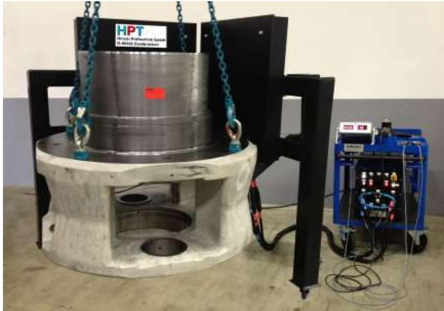
**Figure 4: Non-contact MT-testing and demagnetization of a planet-wheel carrier with two coils and the Hirsch Multipuls-1003-E2-1 (30,000 A) device**
