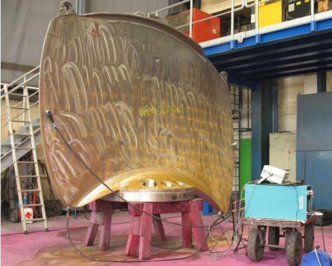
**Figure 2: MT-testing of a blade for a hydroelectric power plant (W= 4.5 m; H= 3.0 m), Hirsch Multipuls-1003-E2-1 device using direct current flow with up to 30,000 A**
