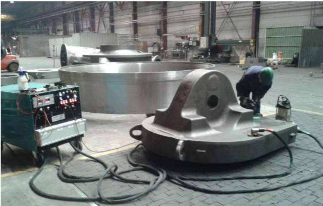
**Figure 6: Mt-testing of a casted component with direct current flow using 3 DC Pulse Technology and the Hirsch Multipuls-1003-E3 (3 x 30, 000 A) device**
