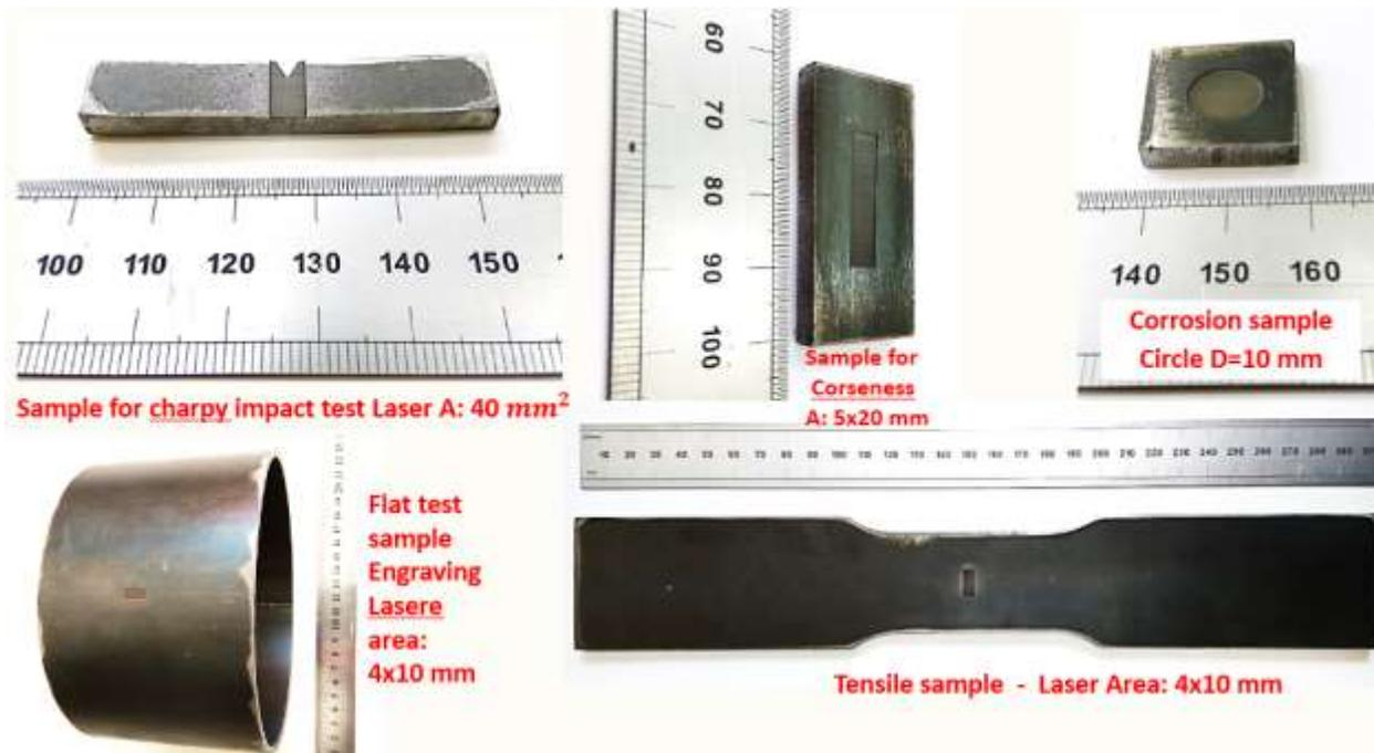
Figure 4. Destructive test samples.
