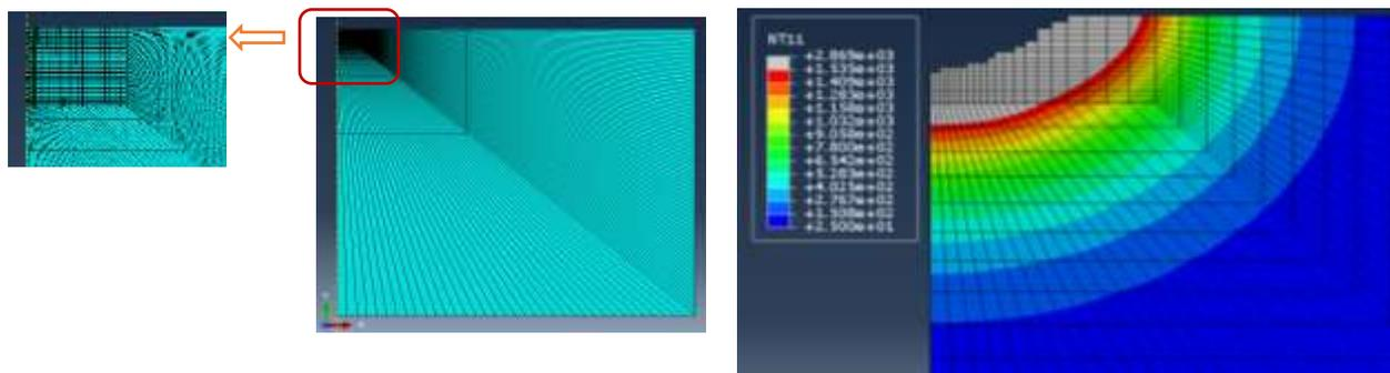
Figure 5. Mesh structure.
