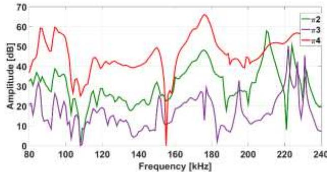
Figure 4. Resonance ultrasound spectra for samples ( $\pi_2$ ,  $\pi_3$ ,  $\pi_4$ )
