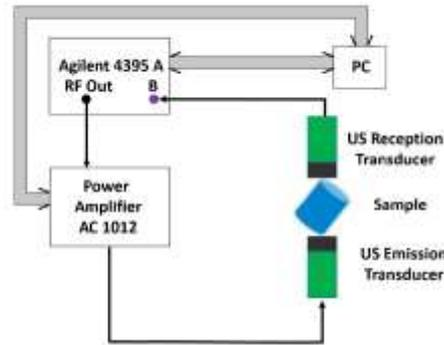
Figure 1. Experimental set-up for RUS-schematic block diagram
