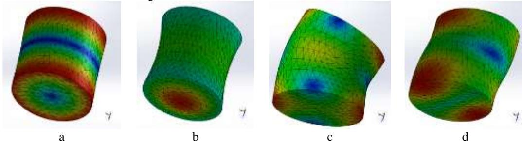
Figure 5. Resonant modes for sample  $\pi_2$ : (a) extensional mode,  $f=163$  kHz; (b) extensional mode,  $f=185$  kHz; (c) flexural mode  $f=208$  kHz; (d) flexural mode  $f=214$  kHz.
