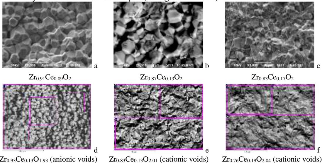
Figure 2.  $\text{Zr}_{1-x}\text{Ce}_x\text{O}_2$  micrography: SEM (a-c); EDX determined (d-f)
