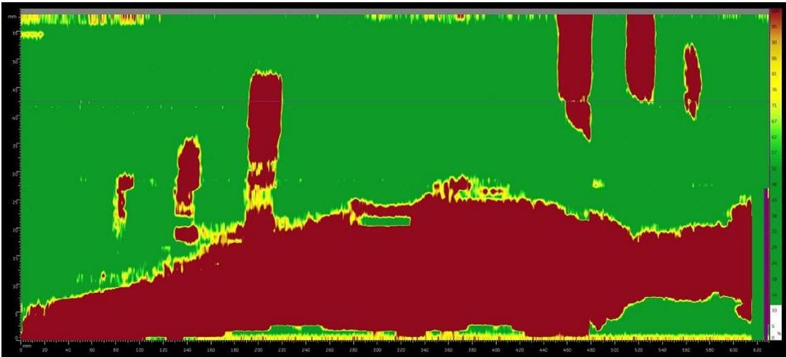
**Figure. 6. C-Scan image of a titanium composite material combination. Areas displayed in red correlate with areas in which either bare titanium was present (red area starting from the lower edge) or the position of artificial defects which have been placed in the adhesive layer.**
