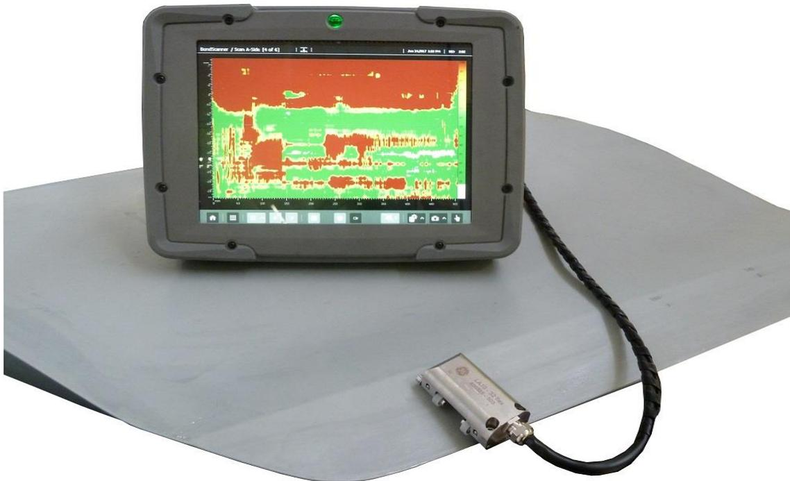
**Figure. 5. Inspection system for adhesive joints. The inspection system consists of the MentorUT ultrasound inspection instrument and an array probe suited to the inspection part.**
