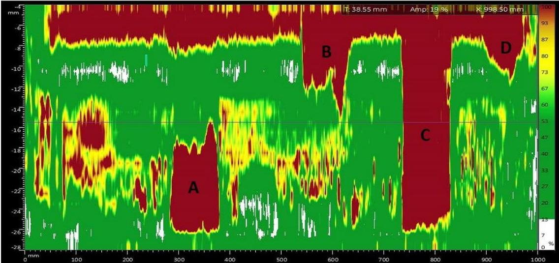
Figure 3. C-Scan Image of a hemming joint. The C-Scan is strongly scaled, actual scan length is about 1000mm. Areas displayed in red correlate with areas in which no adhesive is present in the hemming while areas displayed in green image the distribution of the adhesive in the hemming.
