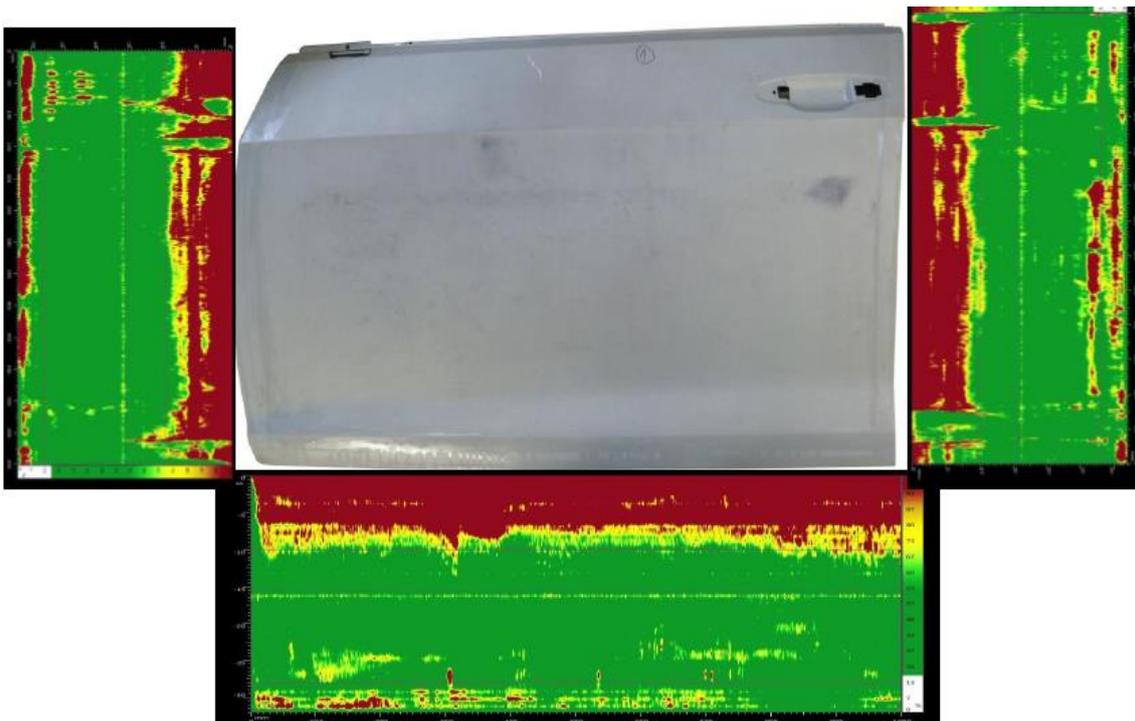
Figure 4. C-Scan images of car door hemming. The C-scans are strongly scaled. The ultrasonic C-Scans represent the distribution of the adhesive in the different hemming on the inspected car door.
