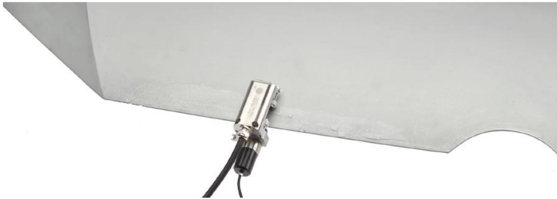
**Figure. 2. Inspection of an engine hood with a flexible linear array in direct contact.**
