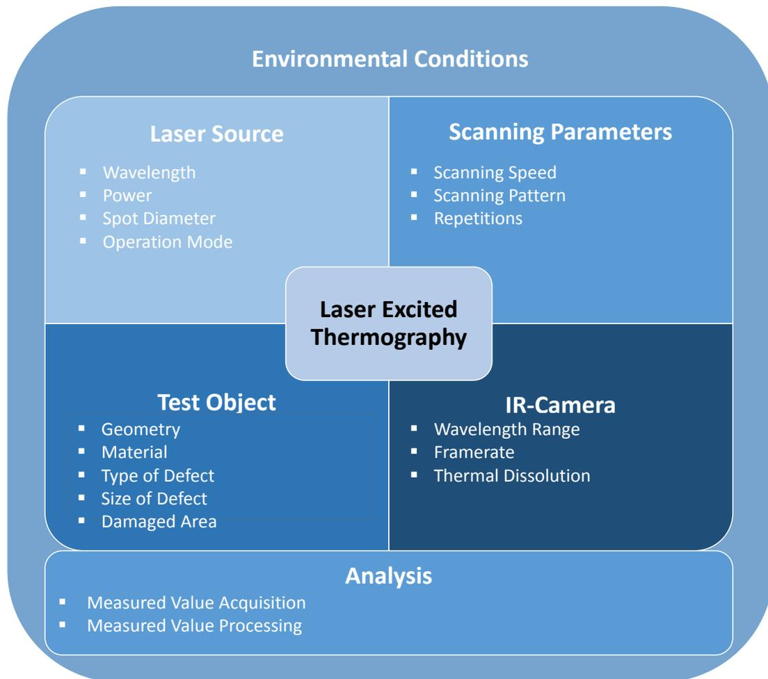
**Figure 1: Overview of parameters that influence the results of active thermography using a scanning laser process as excitation source**
