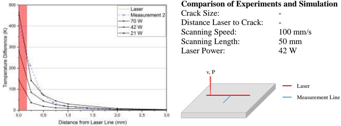
**Figure 3: Exemplary comparison of experimental data and simulation results for definition of heat source**
