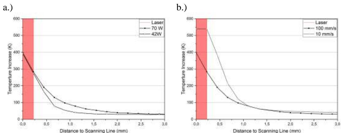
**Figure 2: Influence of process parameters on resulting temperature increase on a measurement line in on one side of the laser source: a.) Laser power and b.) Scanning speed**
