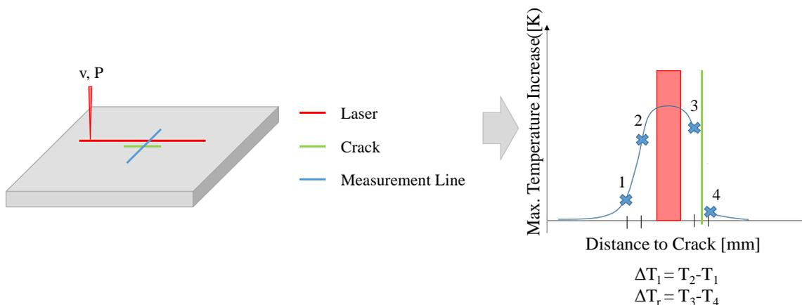
**Figure 4: Definition of temperature differences based on reference points on both sides of the laser source**
