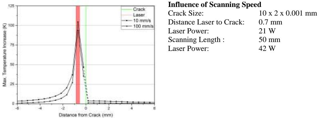
**Figure 5: Influence of scanning speed on the maximum temperature increase**
