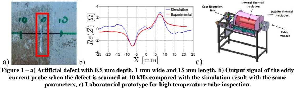
Figure 1 – a) Artificial defect with 0.5 mm depth, 1 mm wide and 15 mm length, b) Output signal of the eddy current probe when the defect is scanned at 10 kHz compared with the simulation result with the same parameters, c) Laboratorial prototype for high temperature tube inspection.
