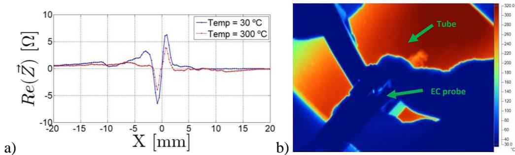
Figure 2 – a) Output signal of the eddy current probe when the defect is scanned at 12 MHz at room temperature and at 300° C, b) Thermographic image of the test.
