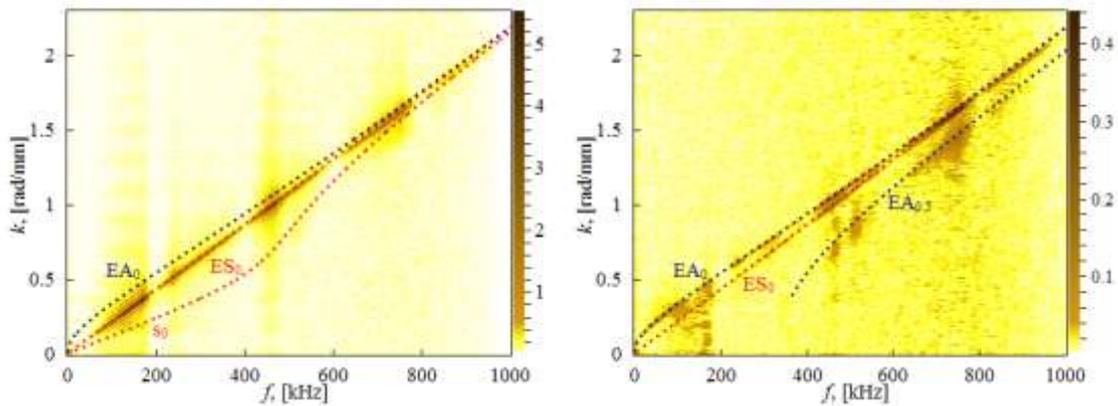
Figure 5. Experimental verification: WFA for pulse loading with theoretical dispersion curves
