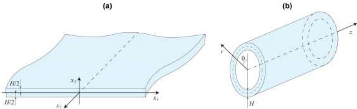
Figure 1. Geometry of the problem: (a) semi-infinite plate; (b) semi-infinite cylindrical shell
