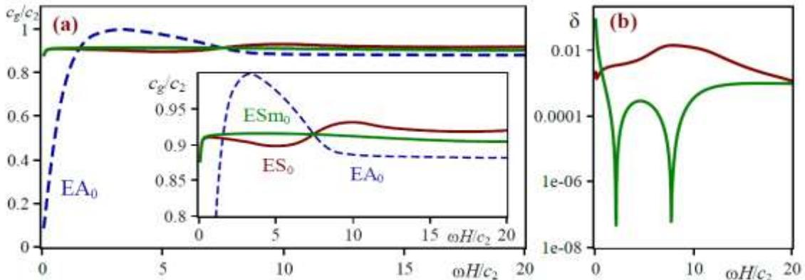
Figure 4. Results for EW in a cylindrical shell: (a) group velocities for the fundamental waves; (b) logarithmical decrement for waves  $ES_0$  and  $ESm_0$
