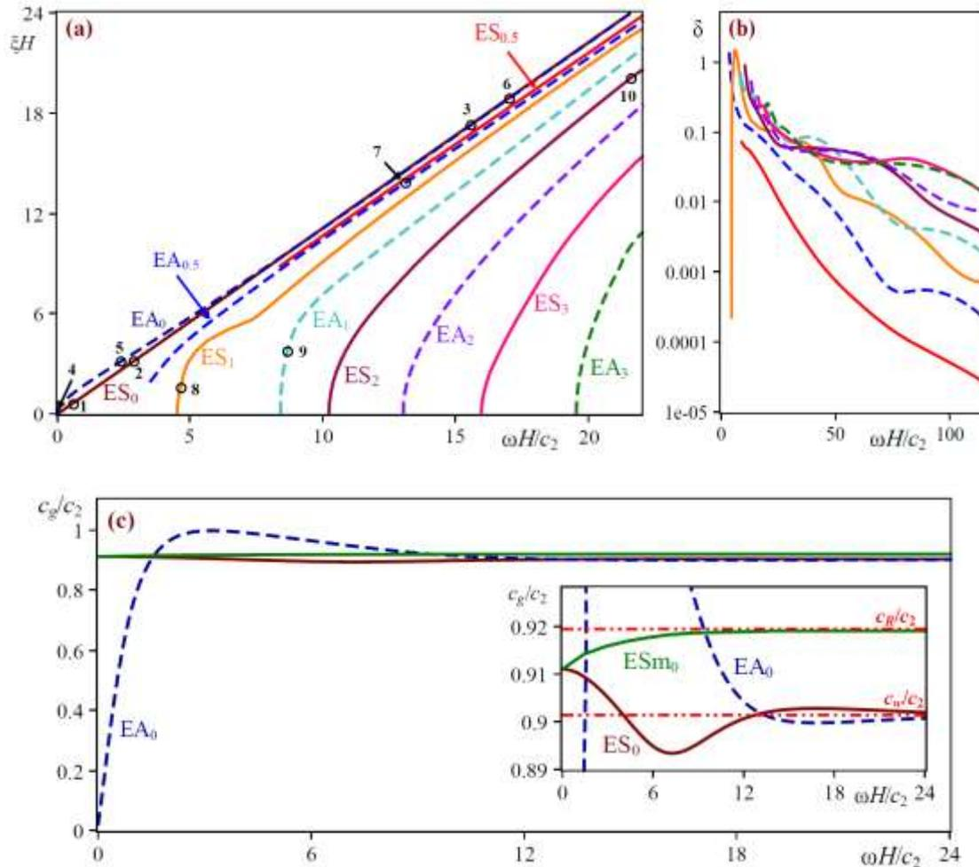
Figure 2. Edge waves in a plate with free faces: (a) dispersion curves; (b) logarithmical decrement; (c) group velocities for fundamental waves
