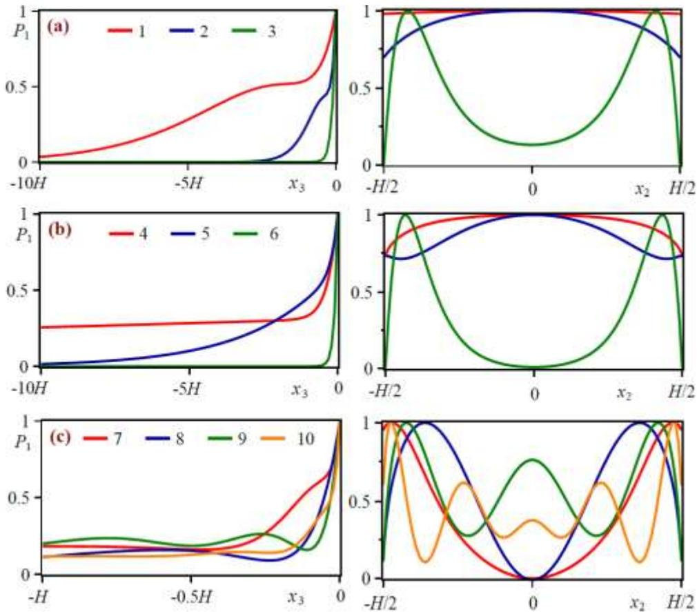
Figure 3. Density of the energy flux along the edge corresponding to the points indicated in Figure 2,*a*: (a) wave  $ES_0$ ; (b) wave  $EA_0$ ; (c) higher order EW
