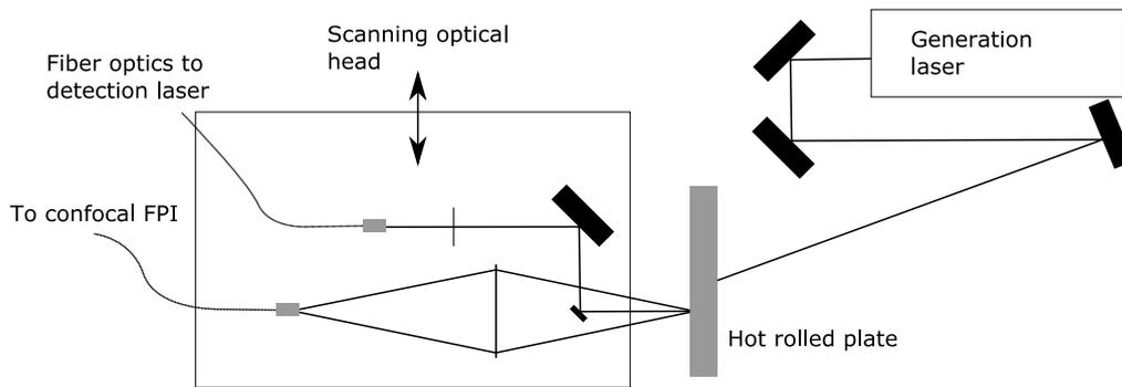
**Figure 3. Simplified representation of the laser ultrasound setup with its optical detection head mounted on a linear axis (4).**
