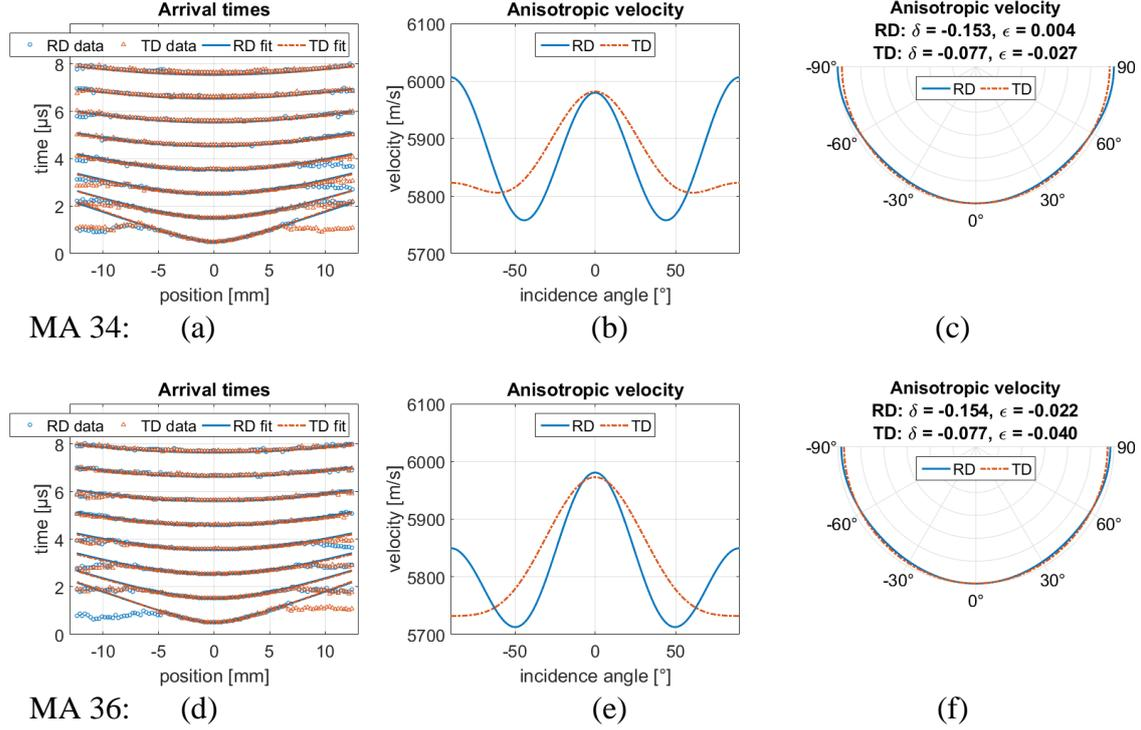
**Figure 4. Results from two Tata Steel MA samples: (a) and (d) the picked data points of arriving wave fronts and fitted anisotropic hyperbolas in two directions (rolling direction and transverse direction), (b) and (e) the corresponding anisotropic velocities as function of incidence angle, and (c) and (f) the same velocities displayed in a polar plot.**
