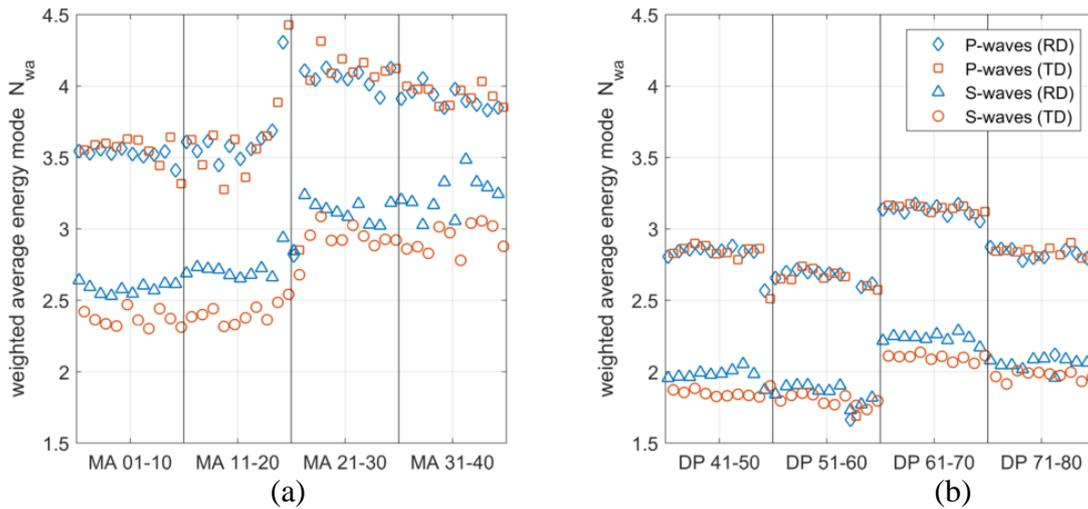
**Figure 6.** The weighted average energies of four sets of Arcelor-Mittal samples: (a) four sets of micro-alloy steel (MA), and (b) four sets of dual phase steel (DP). For each sample, four energies are shown: P-waves in the rolling direction (RD), P-waves in the transverse direction (TD), and S-waves in the rolling and transverse directions.
