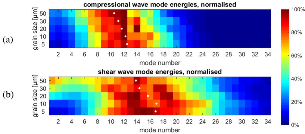
**Figure 5.** The wave mode energies, as function of mode number (horizontal) and grain size (vertical), obtained from numerical simulations. On top (a), the P-wave modes, and on the bottom (b), the S-wave modes. In both figures, the weighted average energy mode is shown as white dots.
