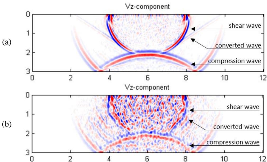
Figure 1. Snapshot from a simulation, at  $0.7 \mu\text{s}$  after a pulse at the surface of the sample. The vertical particle velocity is shown for a sample with an average grain size of  $5 \mu\text{m}$  (a), and of  $50 \mu\text{m}$  (b). The horizontal and vertical axes denote distances in mm. Denoted are the first pressure waves, compressional waves and a mode converted wave.
