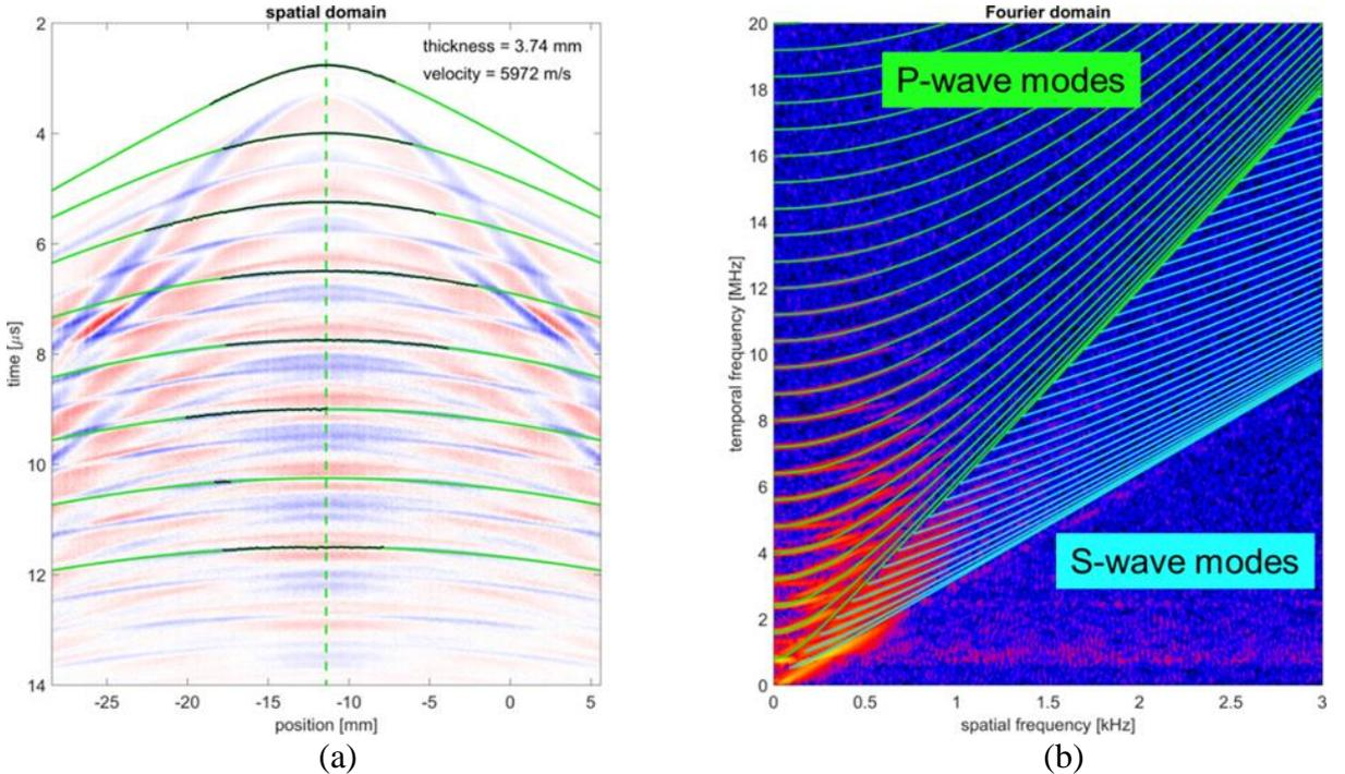
**Figure 2. (a) Recorded data, with tracked compressional waves (black) and overlaid hyperbola estimations (green), which provide an estimation for the sample thickness and compressional wave velocity. (b) The locations of the P-wave modes and S-wave modes, based on the estimated sample parameters, superimposed on the Fourier transformed data (red-blue intensity graph).**
