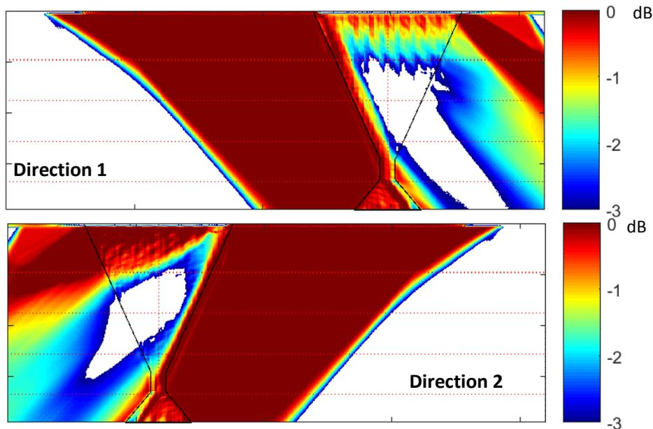
Figure 4. Field overlay for the two scan directions. Refraction angle =  $45^\circ$ . Threshold = -3 dB.
