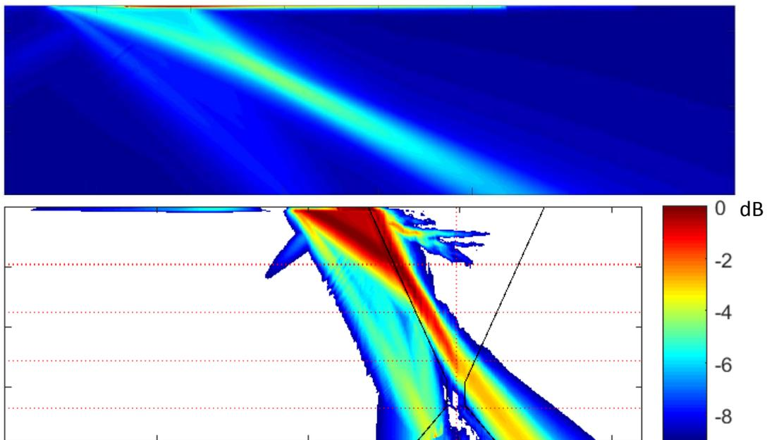
Figure 3. Above: Reference field in parent metal. Below: Computed field normalised by reference field corresponding to the position C on Figure 2. Refraction angle = 45°. Threshold = -9 dB.
