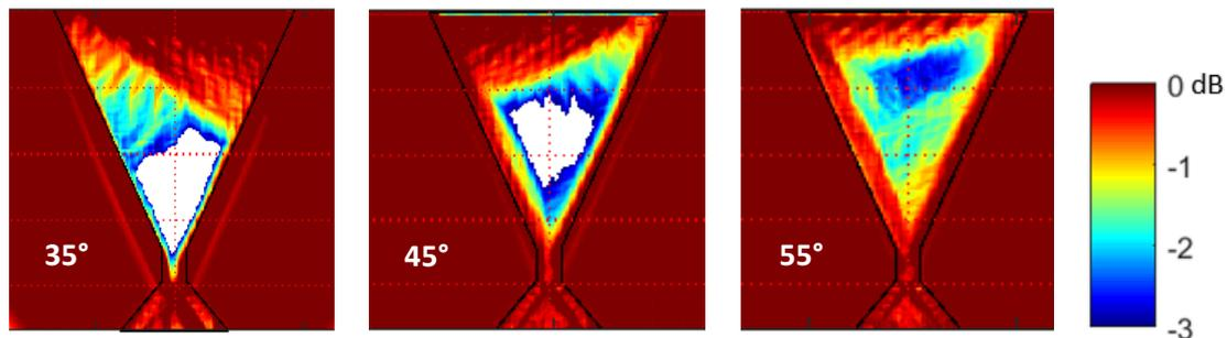
**Figure 5. Field overlays with both directions at the different refraction angles. Threshold = -3 dB.**
