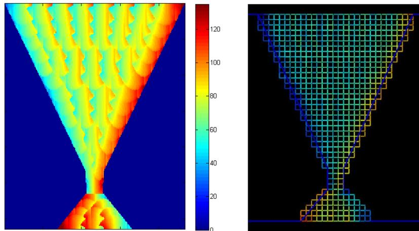
**Figure 1. Weld cartography with grain orientation obtained with MINA model (left: cartography directly computed with MINA; right: average orientations on small squares implemented in ATHENA code)**
