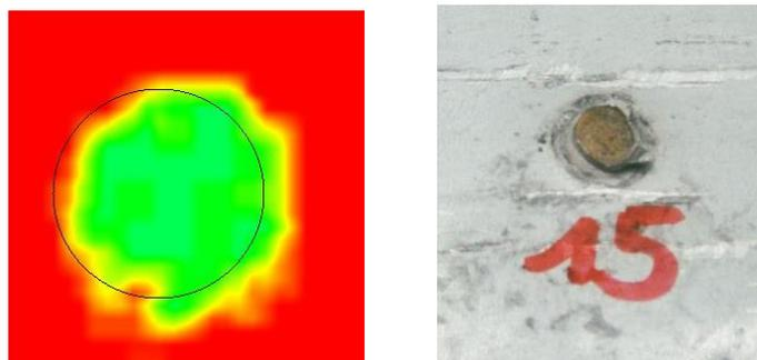
**Figure 3. representative result for steel 0.7/0.8 mm (Left: ultrasonic inspection result; Right: destructive testing result)**
