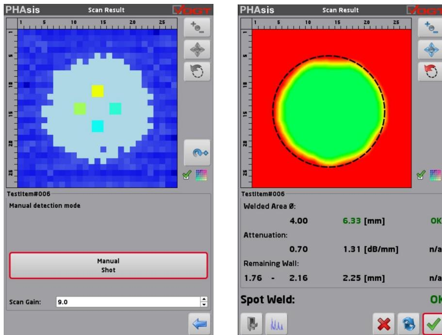
Figure 2. Left: Live-C-Scan for positioning and vertical focussing of the probe on the spot weld surface; Right: Automatically created evaluation proposal
