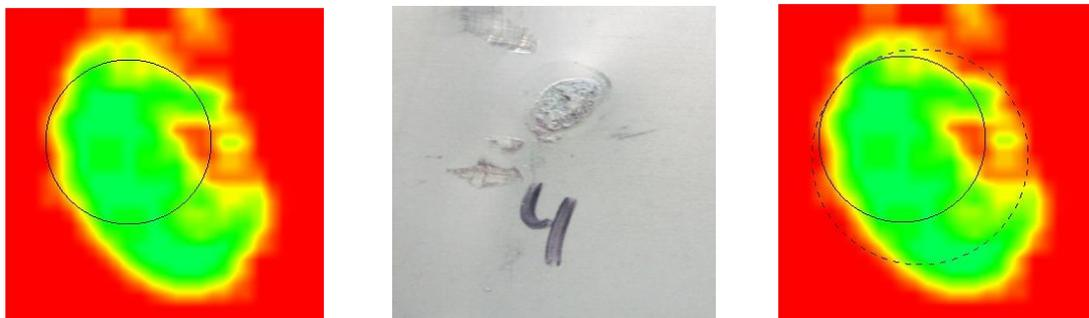
**Figure 4. representative result for aluminium (Left: ultrasonic inspection result; Middle: destructive testing; Right: manual change of ultrasonic inspection result)**
