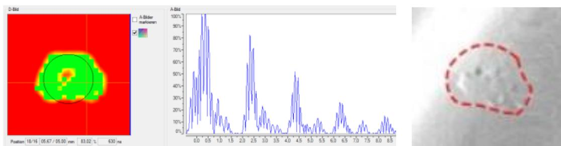
**Figure 5. Left: Ultrasonic inspection d-scan incl. an exemplary a-scan; Right: CT image**
