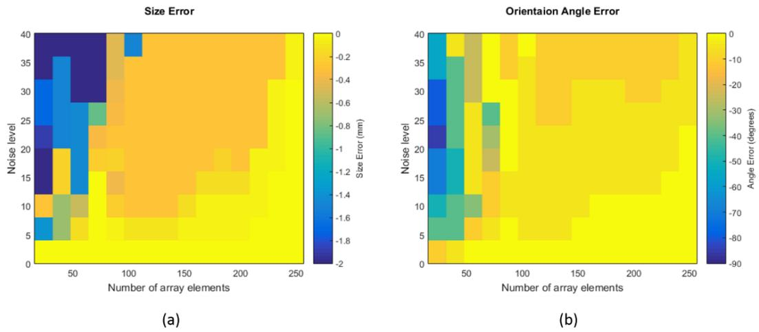
**Figure 1. Array performance in characterising (a) size and (b) orientation angle of a simulated crack against number of elements and noise level. The simulated crack has a size of 0.5 mm and is oriented at 60° from the array.**
