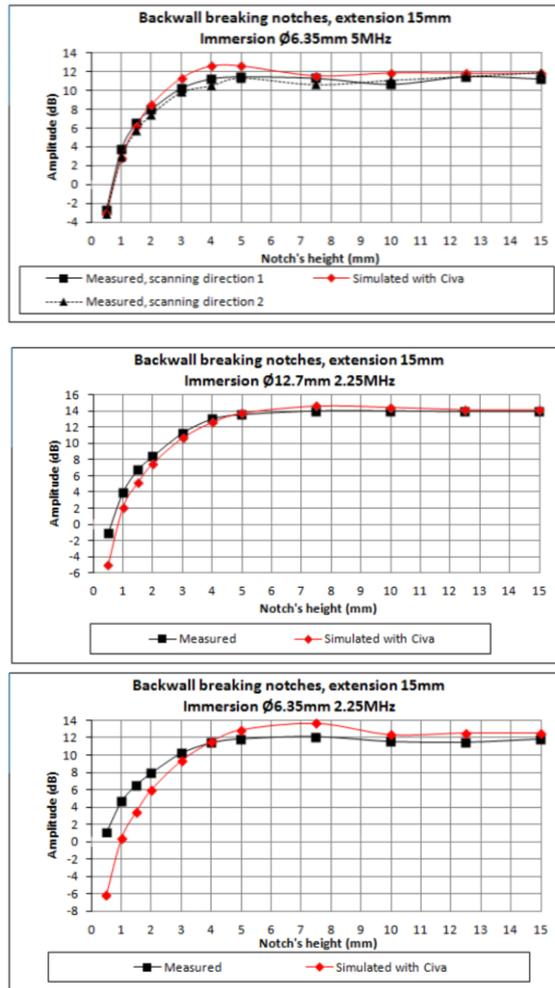
Figure 2. Graphs of the simulated and experimental amplitude measured on the corner echoes as a function of the flaw height and for 3 immersion probes (from top to bottom: 5MHz  $\varnothing 6,35$  mm probe, 2.25MHz  $\varnothing 12,7$  mm probe, 2.25MHz  $\varnothing 6,35$  mm probe)
