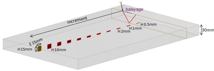
Figure 1. Ferritic steel mock up including vertical notches with various heights
