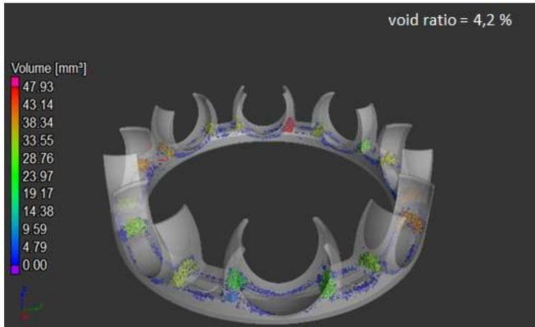
**Figure 1. X-ray Computed Tomography: location and dimensioning of porosities**
