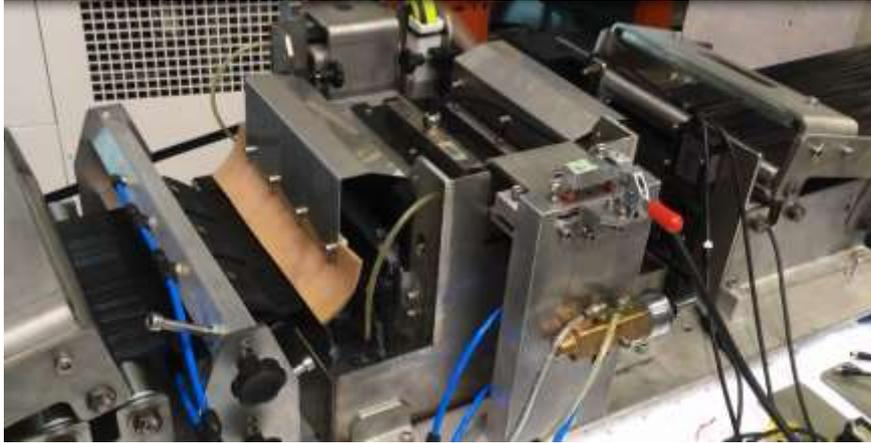
**Figure 2. Online ultrasonic phased array inspection system of pultruded thermoplastic tapes**
