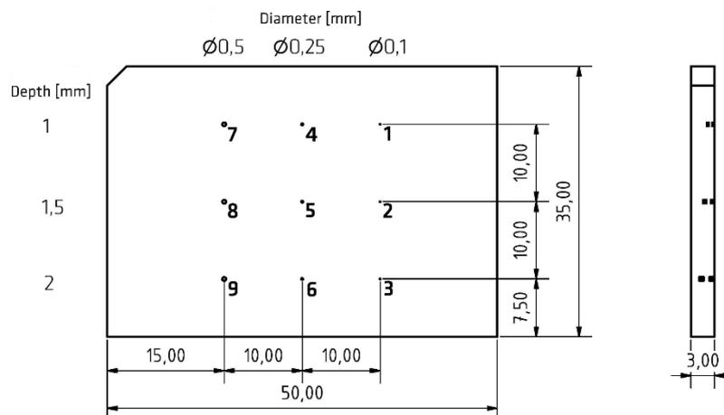
**Figure 2: Calibration block for plate type specimen**
