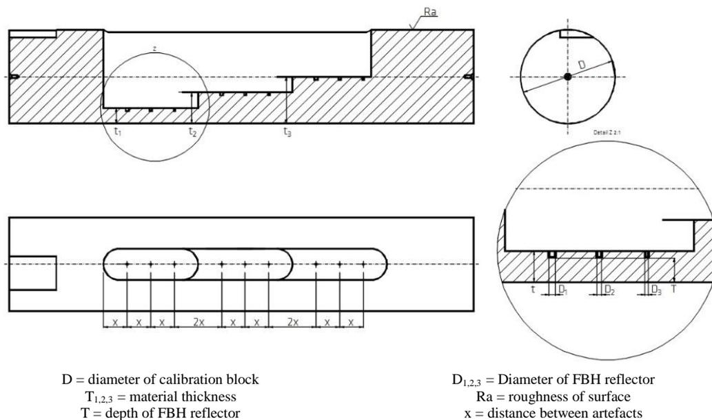
**Figure 1: Reference block for bar type specimen (in style of SEP 1927)**
