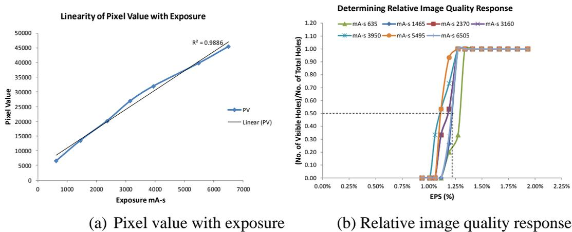
Figure 4: Linearity of pixel value with exposure (a) relative image quality response (b)
