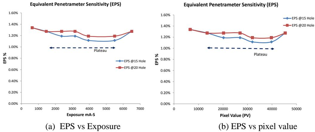
Figure 3: Equivalent penetrameter sensitivity (EPS) vs exposure (a); pixel value (b)
