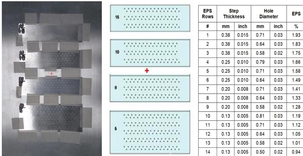
Figure 2: EPS and aluminium (Al) absorber plate setup
