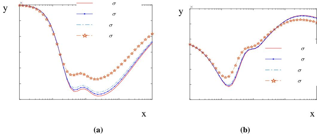
Figure 2. Effects of different ( $\Delta\sigma$   $\Delta\mu$   $\Delta t$   $\Delta l$ ) on both real part (a) and imaginary part (b) of conductivity sensitivity of the referred point ( $Re(\Delta L)/\Delta\sigma$  and  $Im(\Delta L)/\Delta\sigma$ )
