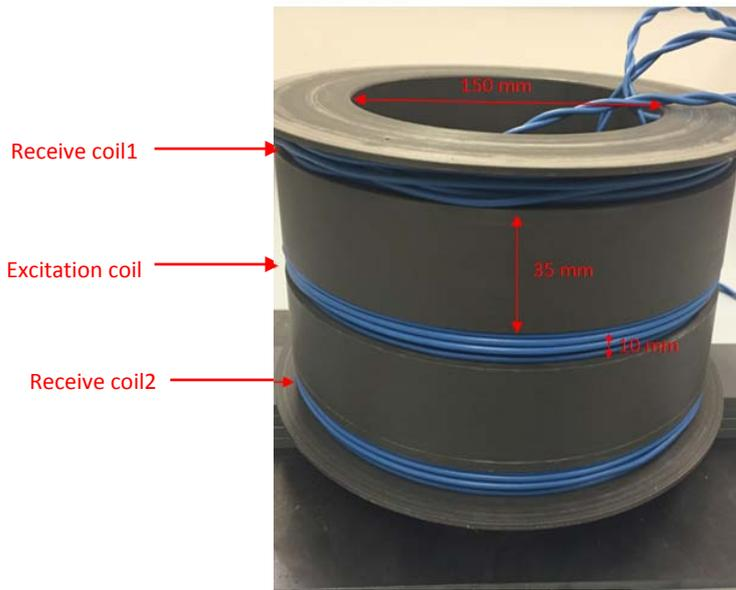
**Figure 1. Sensor configuration**
