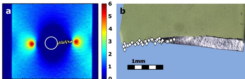
**Fig 1. Crack tip positions in the simple coupon mapped using the automated algorithm: a) overlaid on final normalised TSA signal magnitude data (specimen width 40 mm); b) overlaid on final crack morphology (inset of right side of specimen).**
