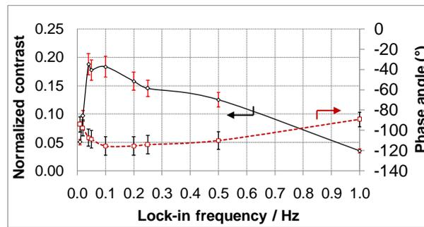
**Figure 4. Effect of the modulation frequency on normalized contrast computed over the defected area and phase angle plot (errors bars showing  $\pm$  standard deviation on three repeated measurements) ( $f_c=25$  kHz,  $P\%=12$ ,  $N=1$ )**
