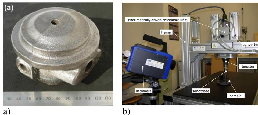
**Figure 1. a) cast iron turbo housing sample (type 1) and b) experimental set-up for ultrasound excited thermography**
