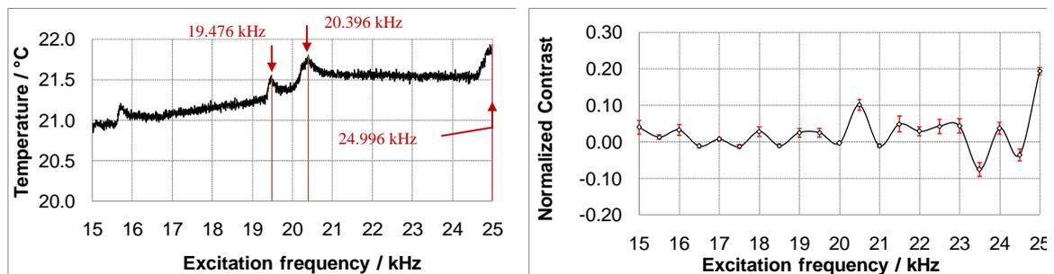
**Figure 2. a) thermo-acoustic spectrum after frequency wobbling and b) normalized contrast ( $\pm$  standard deviation) as a function of the excitation frequency measured in lock-in mode with 0.05 Hz amplitude modulation ( $N=1$ ,  $P\%=12$ )**
