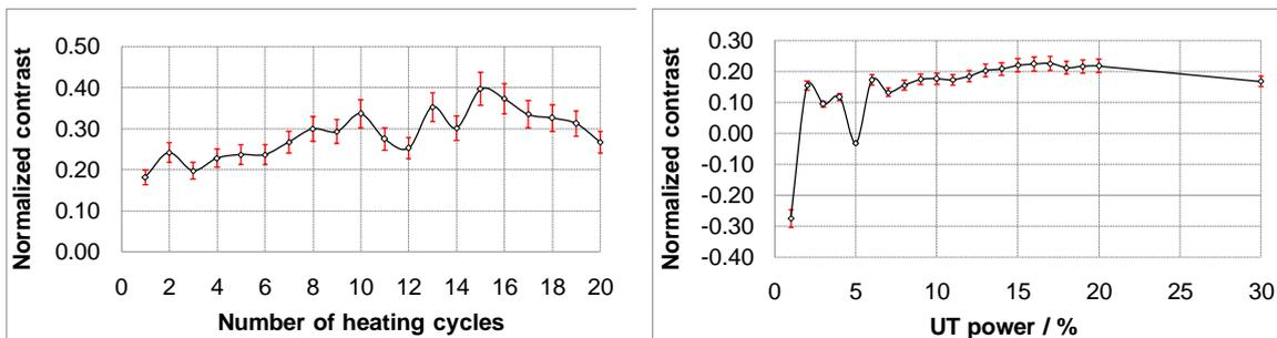
**Figure 3. a) effect of the number of heating cycles on defect detection ( $f_m=0.05$  Hz,  $f_c=25$  kHz,  $P\%=12$ ) and b) normalized contrast as a function of percentage ultrasound power (errors bars showing  $\pm$  standard deviation on three repeated measurements) ( $f_m=0.05$  Hz,  $f_c=25$  kHz,  $N=1$ )**
