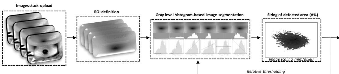
Fig. 7. Flow chart of the algorithm used for defect size assessment
