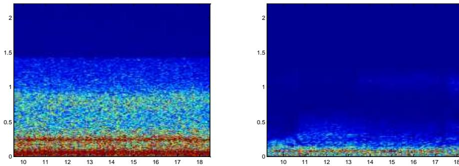
Figure 5. Spectrograms of a failure fan (left) and a same type normal fan (right)
