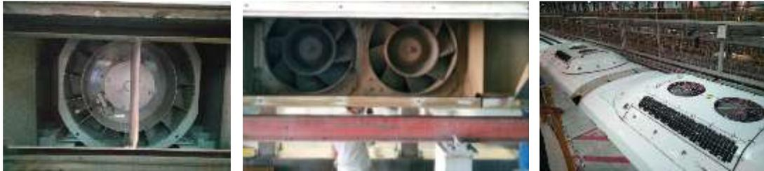
**Figure 1. Converter fan of CRH 380A (left), Air conditioning fan (middle) and Evaporating fan on the roof (right) of CRH380B**
