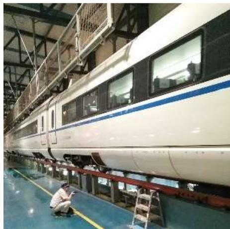
**Figure 1. Manual inspection zone of EMU acceptance inside maintenance depot: condition check employing eye, ear and nose**
