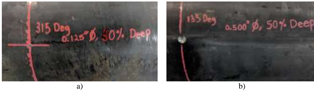
Figure 7. Machined defects D1.A and D1.B
