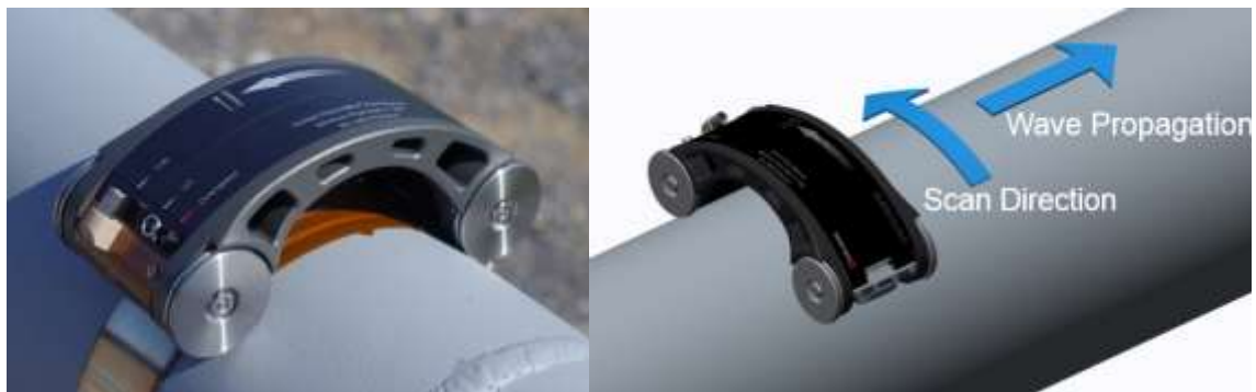
Figure 5. a) MRUT MS Scanner placed on a MS Strip b) Circumferential scanning sending the waves both sides in the axial direction
