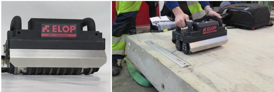
**Figure 1. The handheld scanner unit connected to the external electronics box inside the backpack. The cable features robust, waterproof connectors at both ends for rugged outdoor use.**
