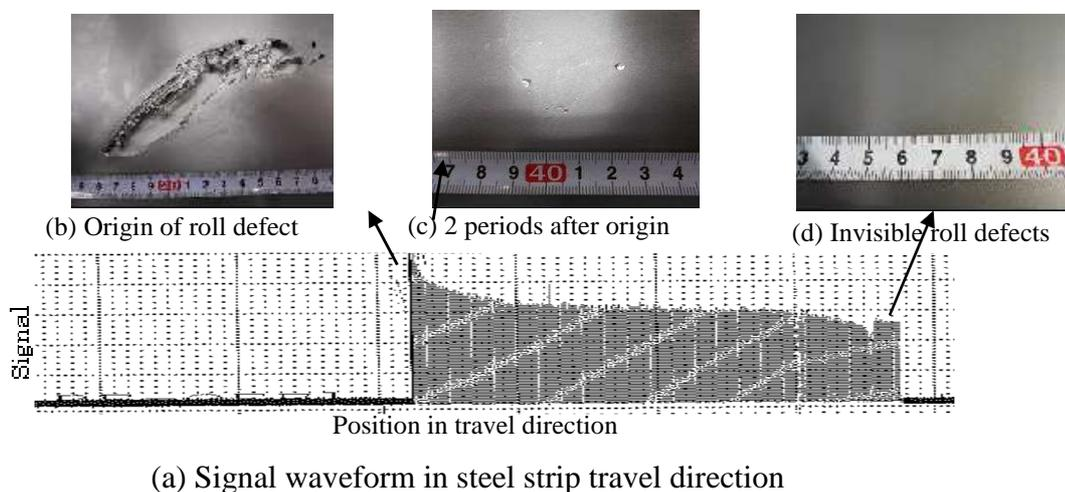
(a) Signal waveform in steel strip travel direction
