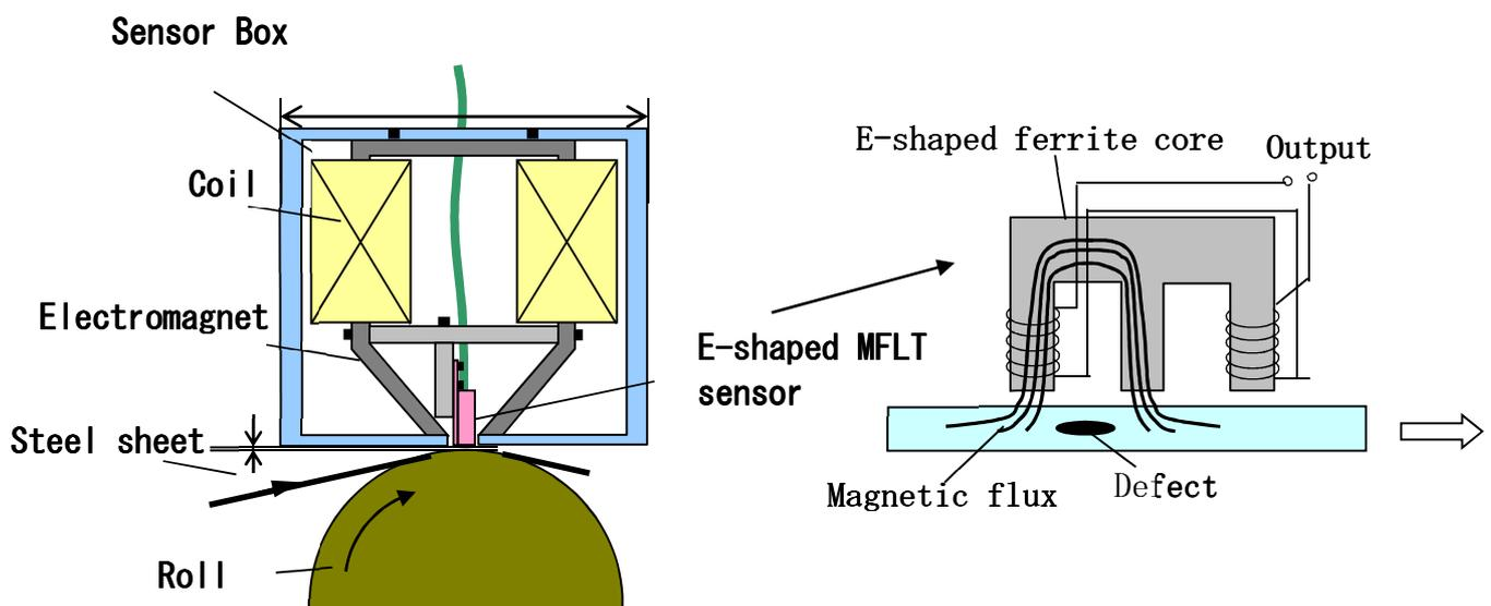
Fig. 1 Schematic of on-line measurement system
