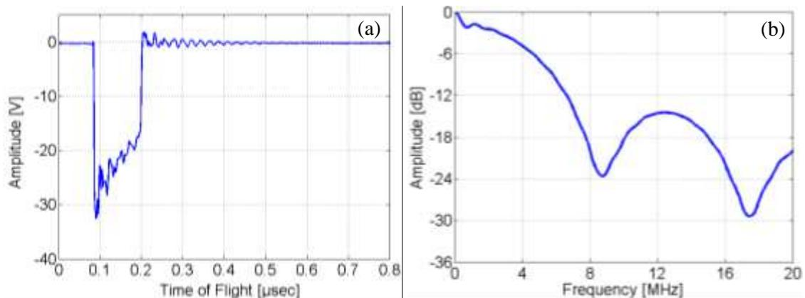
Figure 2. Excitation waveform used for the ultrasonic pulse-echo measurements: (a) time-domain signal, (b) Fast Fourier Transform of the excitation signal.
