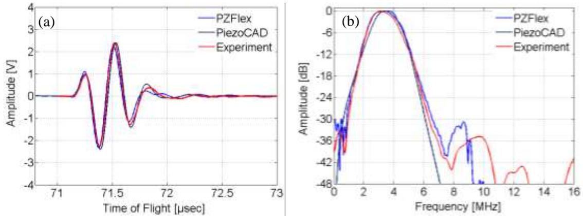
**Figure 3. Comparison between the experimental, PZFlex and PiezoCAD simulated ultrasonic pulse-echo response of the 1-3 piezocomposite based ultrasonic sensor: (a) time-domain signal, (b) normalized Fast Fourier Transform of the signal.**
