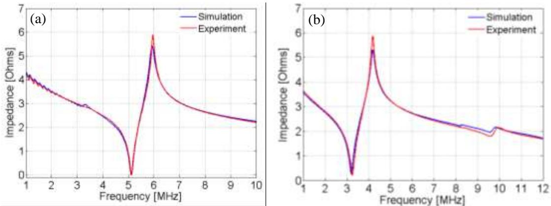
Figure 1. Comparison between the experimental and PZFlex simulated electrical impedance: homogeneous piezoceramic material, (b) 1-3 piezocomposite material fabricated using the dice-and-fill technique.
