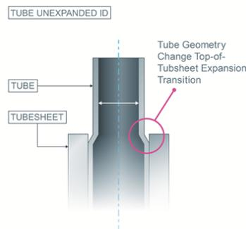
**Figure 1. Cross section of Top-of-Tubesheet Expansion Transition Region**
