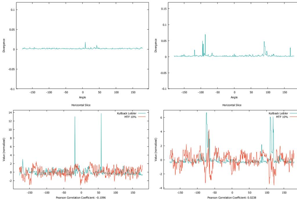
**Figure 6: Angle dependant evaluations. On the top: Evaluation of the clean slice (left) and the slice with the obstruction object. The influence of the object is clearly measurable by the Kullback-Leibler divergence by several orders of magnitude. On the bottom: comparison with the directional MTF, left without and right with obstructing object. For this comparison, the signals are normalised to zero mean and standard deviation of one.**
