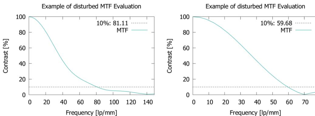
**Figure 5. Directional modulation transfer function, including an obstructing object, best (left) and worst (right) evaluation from the same slice, over both spheres. The curves are more dissimilar than in the example without the obstructing object.**
