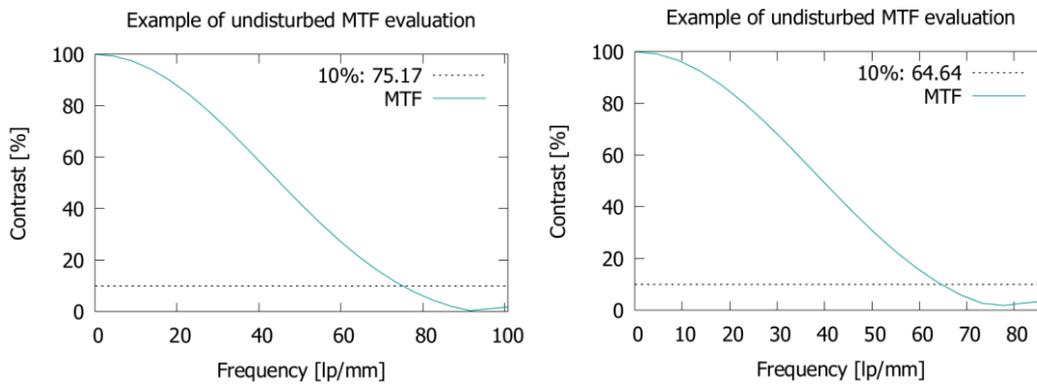
**Figure 4. Directional modulation transfer function, without obstructing object, best (left) and worst (right) evaluation from the same slice, over both spheres. The two measurements are close to each other.**
