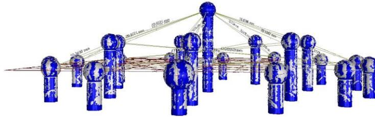
**Figure 1. Example of the influences of materials. The reconstruction's extracted surface of a gauge is fitted to its ideal mesh. Noteworthy are the stripes on the spheres which are aligned with the other parts of the gauge.**
