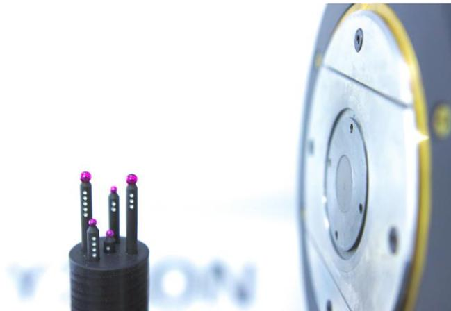
**Figure 2.** Gauge used for the experiments in front of the microfocus X-ray tube. The spheres consist of ruby. Only the upper two spheres are analysed in this survey.
