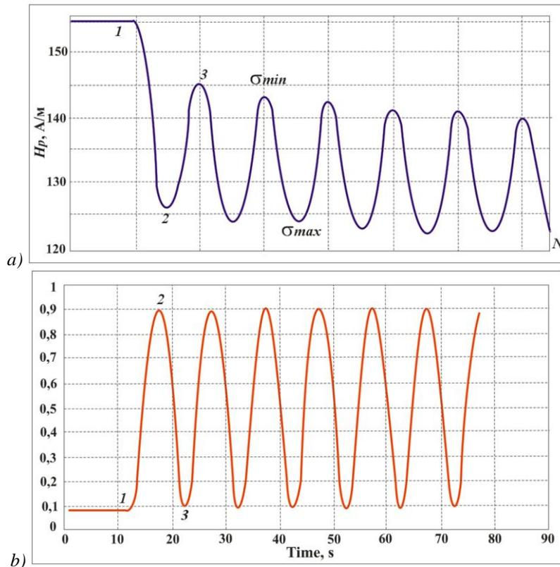
Figure 2. Curve of self-magnetic field  $H_p$  intensity variation during cycling with frequency of 0.1 Hz in the tensile loads range from 7.7 MPa to 77 MPa (*a*) vs the mechanical curve (*b*) recorded on the testing machine:  $N$  – number of cycles
