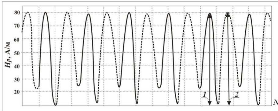
Figure 5. Magnetogram of the specimen's self-magnetic field components  $|\Delta H_a|$  (1) and  $|\Delta H_{rel}|$  (2) variation recorded after 226900 load cycles
