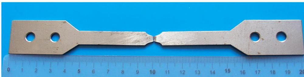
Figure 1. General view of a static and fatigue test specimen
