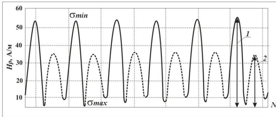
Figure 4. Dependence of the longitudinal magnetic component on the time at the initial stage of the specimen loading (before 100000 cycles):  $N$  – number of load cycles; 1 –  $|\Delta H_a|$ ; 2 –  $|\Delta H_{rel}|$
