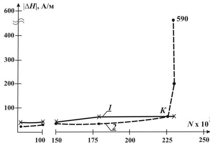
Figure 7. Variation of self-magnetic field components  $|\Delta H_a|$  (1) and  $|\Delta H_{rel}|$  (2) depending on the number of tensile load cycles  $N$ :  $K$  – point of  $|\Delta H_a|$  and  $|\Delta H_{rel}|$  components intersection (equity of values) at  $N=227350$
