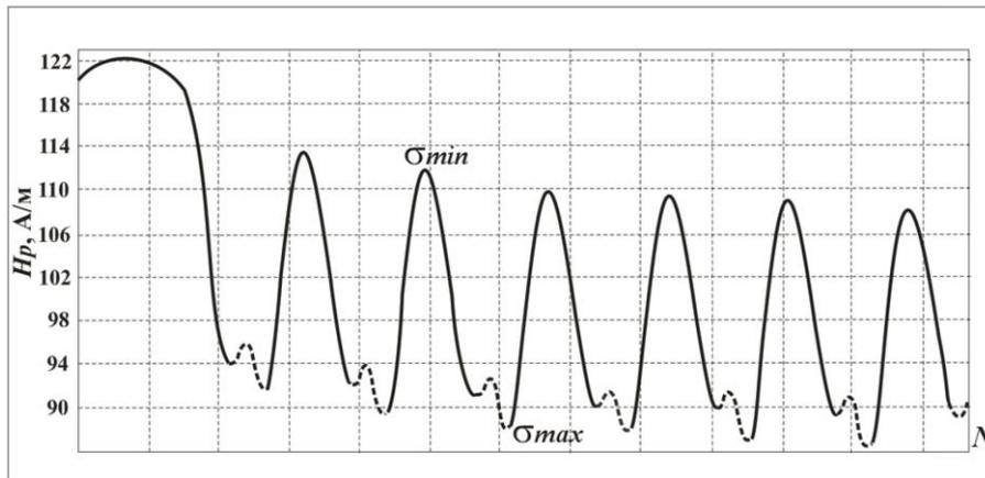
**Figure 3. Curve of the specimen's self-magnetic field intensity variation during cycling with the frequency of 0.1 Hz and maximum load of 156 MPa**
