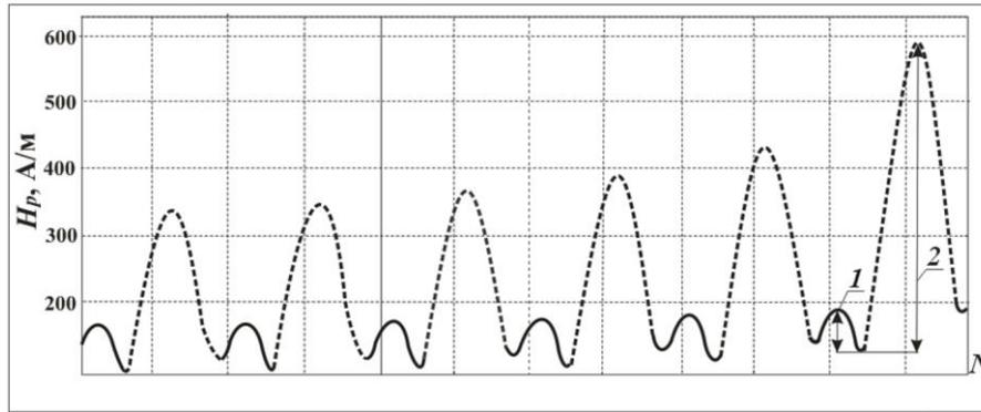
Figure 6. Magnetogram of the specimen's self-magnetic field components  $|\Delta H_a|$  (1) and  $|\Delta H_{rel}|$  (2) variation recorded after 226900 load cycles at the final stage of the specimen failure
