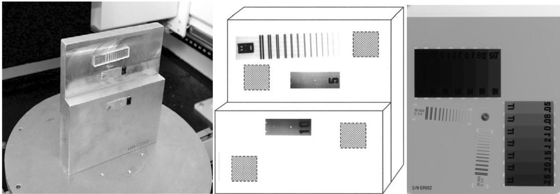
Figure 4. From the left: Picture of the ASTM phantom, drawing of the ASTM phantom, X-ray image of a TAM phantom
