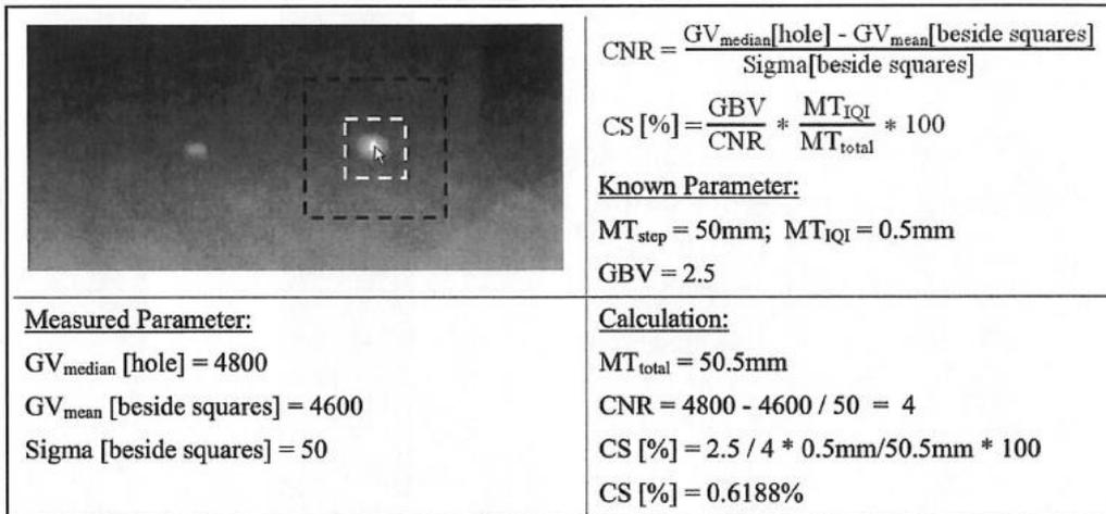
Figure 1. Calculation of CNR values with a hole type IQI
