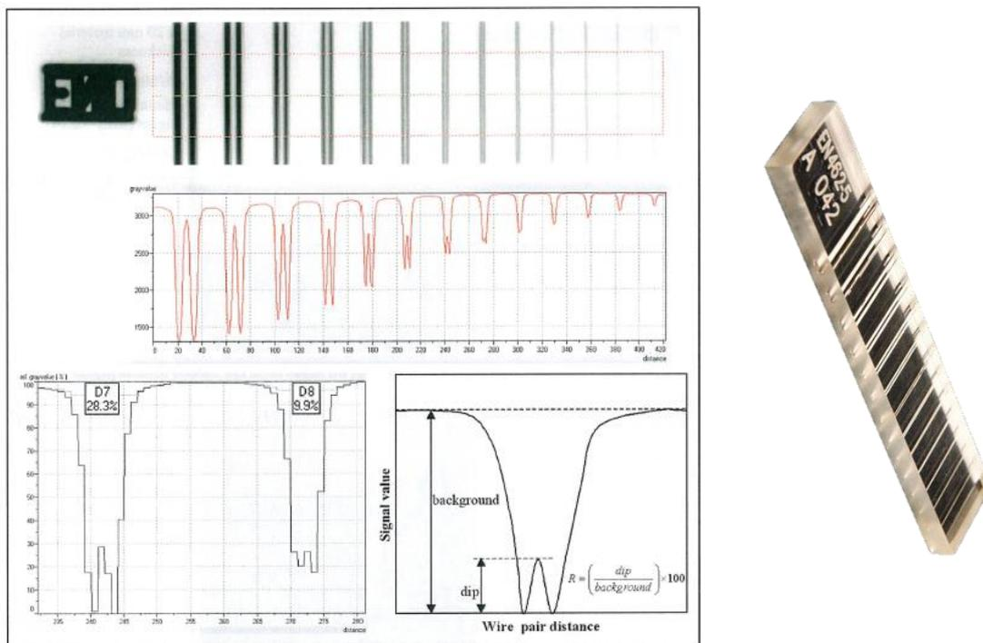
Figure 2. Calculation of Spatial Resolution (SRb) with a Duplex Wire IQI
