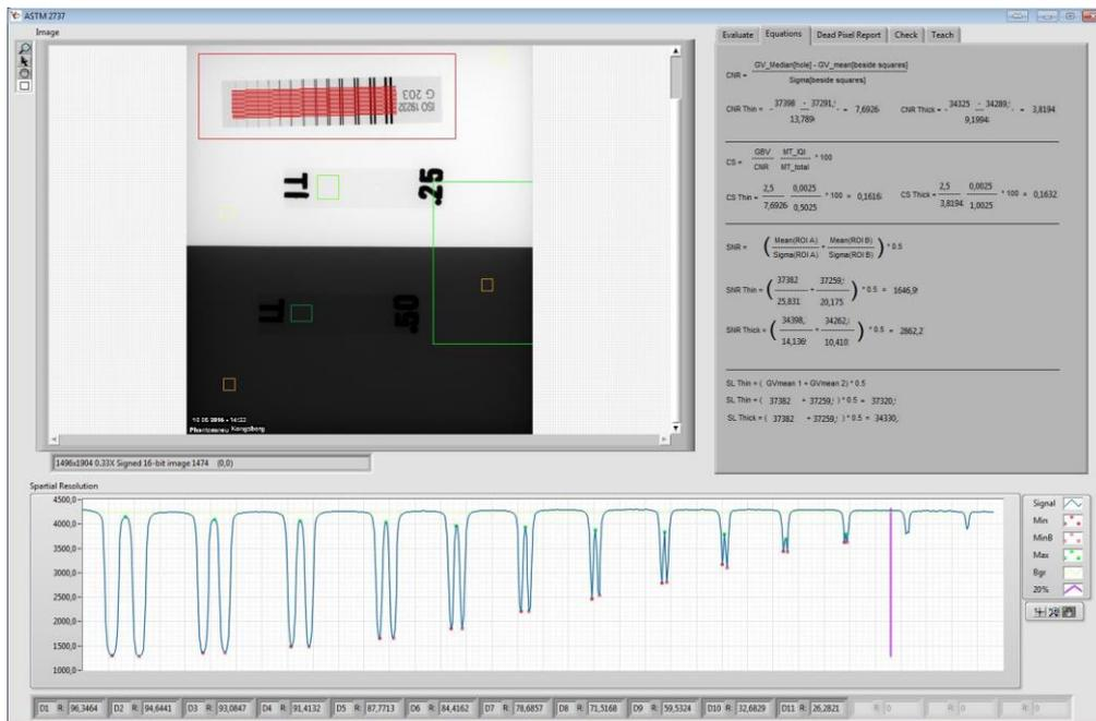
Figure 5. Automatic evaluation of all system performance parameters through the VisiConsult evaluation module.
